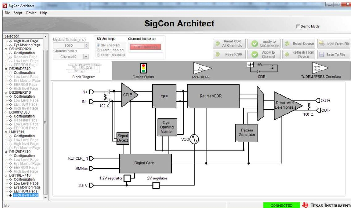
Figure 5. SigCon Architect High Level Page: Block Diagram
