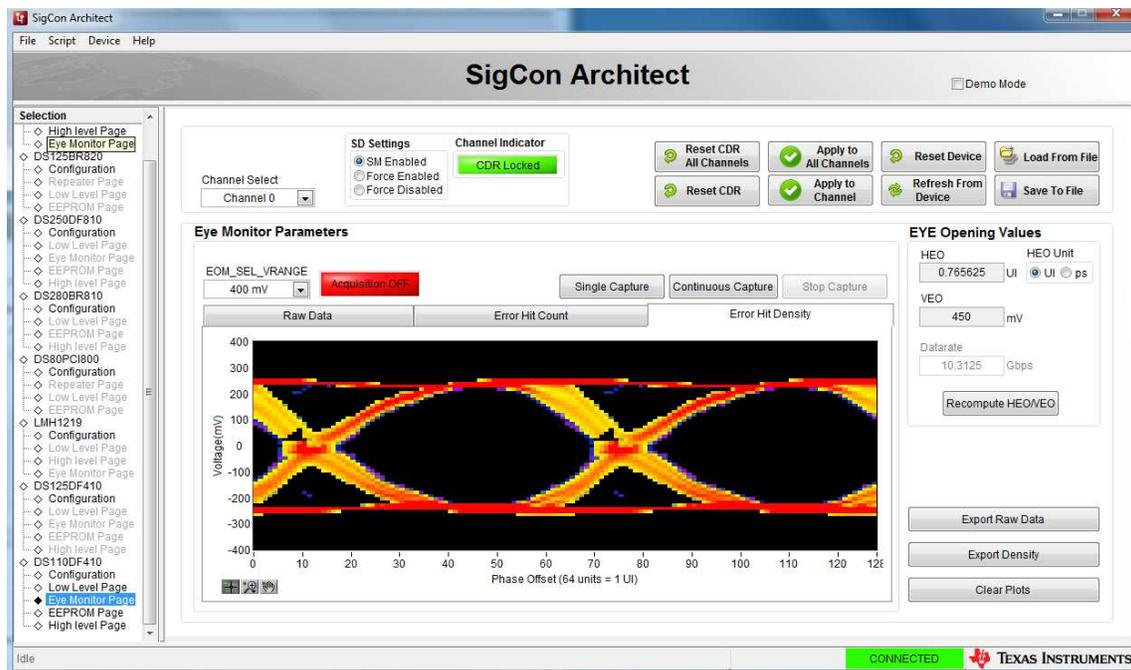
Figure 13. SigCon Architect Eye Monitor Page: Error Hit Density
