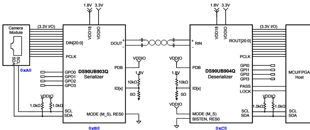
**Figure 6. Example of DS90UB903Q/904Q in Camera Application**
