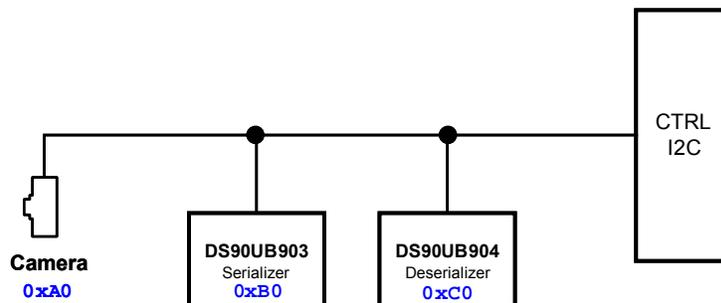
**Figure 7. Virtual device addressing from MCU/FPGA I<sup>2</sup>C controller**
