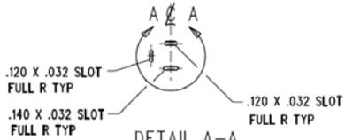
THRU HOLE SLOT - SEE DETAIL A-A
