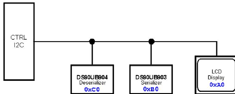
**Figure 5. Virtual device addressing from GPU/FPGA I2C controller**
