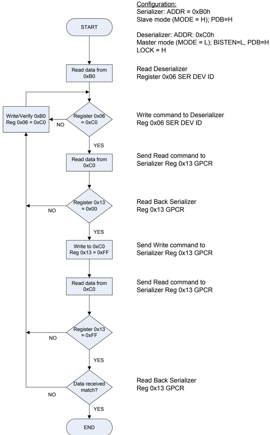
**Figure 5. Bi-directional Control Channel Communication Flowchart in Display Mode**
