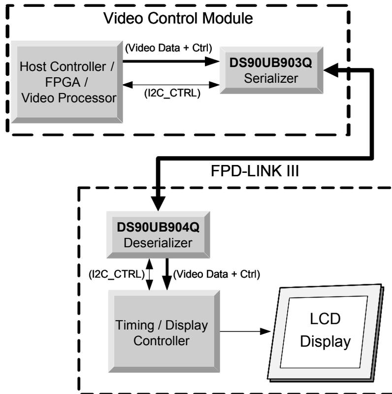
**Figure 2. Typical DS90UB903Q/904Q Display System Diagram**
