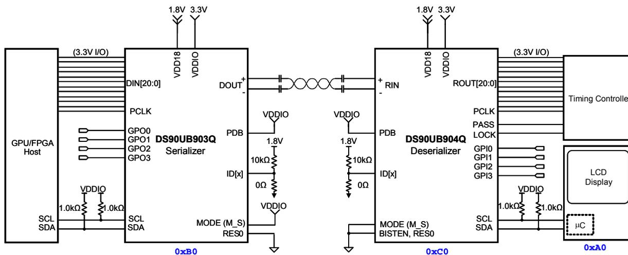
Figure 4. Example of DS90UB903Q/904Q in Display Application
