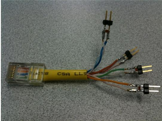
**Figure 2-6. 100 Ohm Terminated Cable for MDI Signal Measurement**
