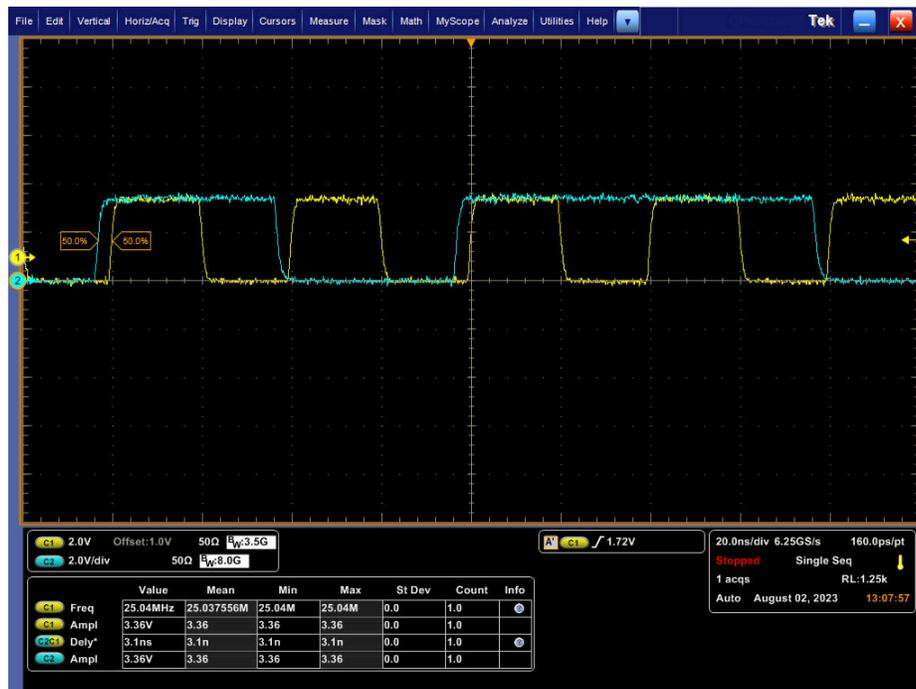
Figure 2-14. RX\_CLK and RX\_D0 Timing in RGMII RX Shift Mode (Yellow Waveform (Channel 1) = RX\_CLK, Blue Waveform (Channel 2) = RX\_D0)
