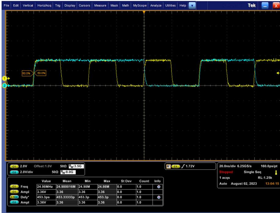
Figure 2-13. RX\_CLK and RX\_D0 Timing in RGMII Align Mode (Yellow Waveform (Channel 1) = RX\_CLK, Blue Waveform (Channel 2) = RX\_D0)
