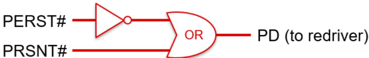
Figure 4-3. PD Control Logic Example with Two Input Signals
