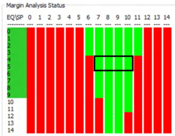
Figure 6-3. Margin Analysis Plot - RX PORT2 (CH3)
