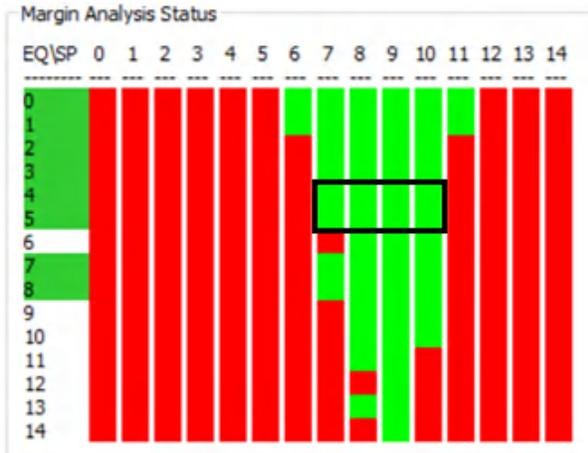
Figure 6-1. Margin Analysis Plot - RX PORT0 (CH1)
