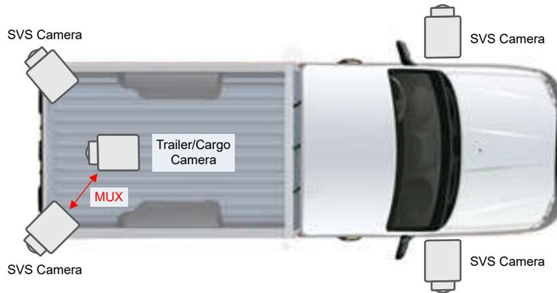
**Figure 1-1. Automotive Application of Multiplexing FPD-Link SerDes**
