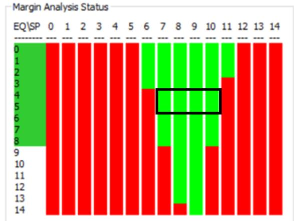
Figure 6-2. Margin Analysis Plot - RX PORT1 (CH2)
