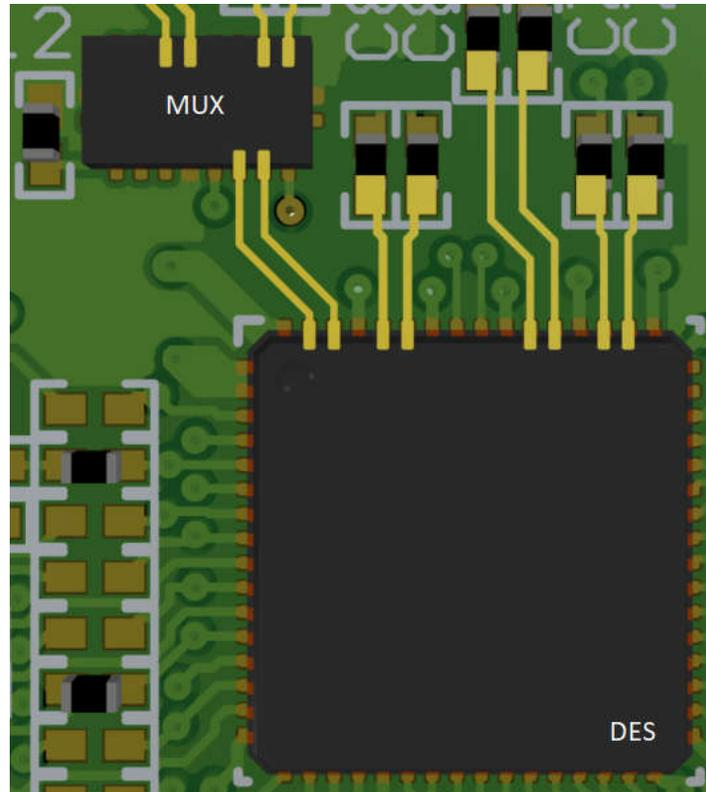
Figure 5-1. Multiplexer and Deserializer Configuration
