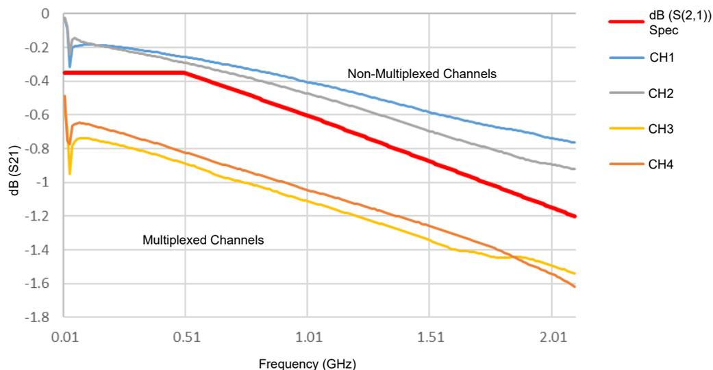
Figure 5-3. Channel Insertion Loss
