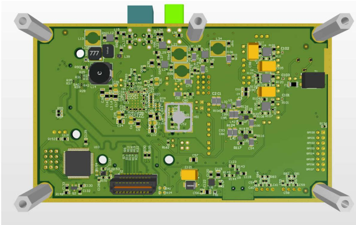
**Figure 3-2. Multiplexing Board Layout - Bottom**
