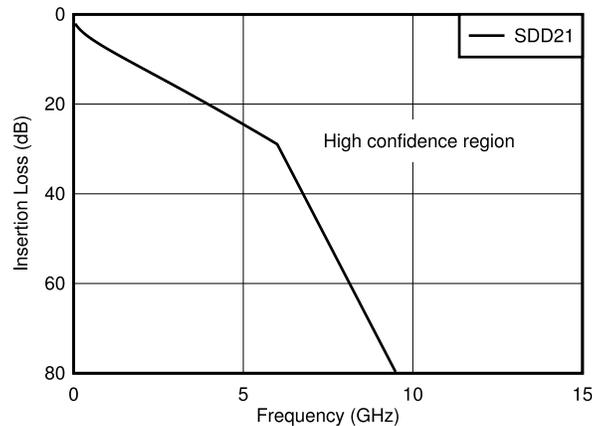
Figure 3-2. Insertion Loss Limit for 10GBASE-KR and 40GBASE-KR4 (IEEE802.3 Annex 69, Figure 69B-5)
