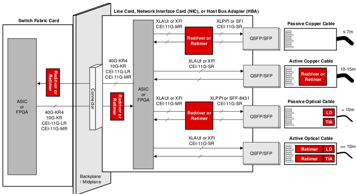
Figure 4-1. Typical Application Use Cases for Signal Conditioning in a 10GbE or 40GbE System
