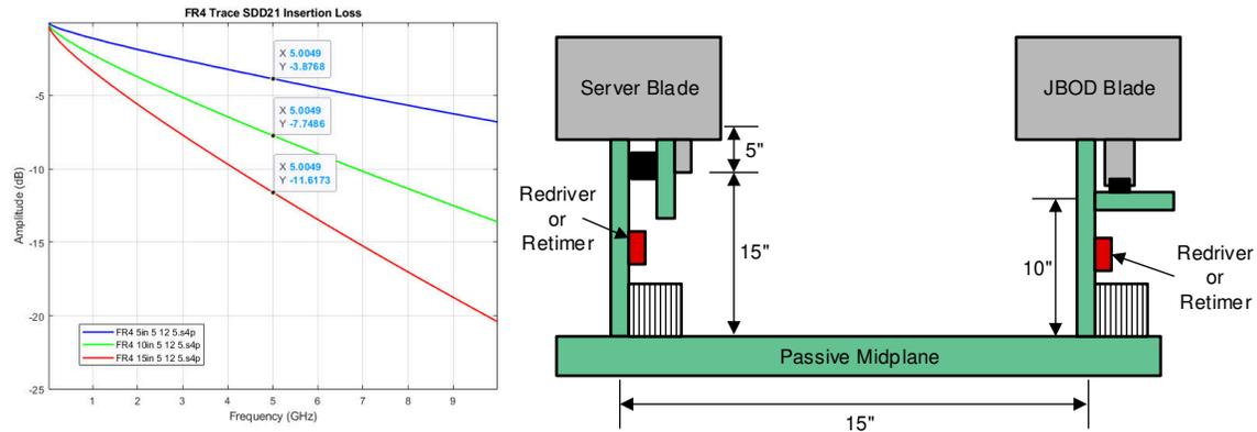
**Figure 2-2. IL Increases with Frequency While PCB Distance Remains the Same**
