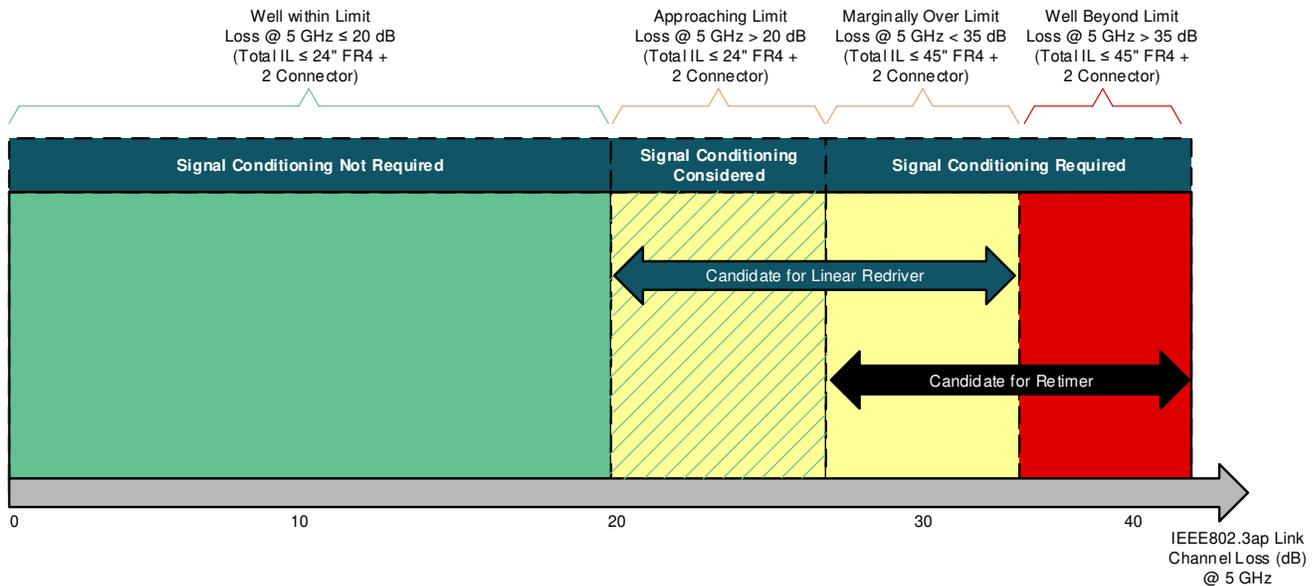
Figure 3-3. Link Budget Example to Determine Redriver Verses Retimer for 10GbE Backplane Applications
