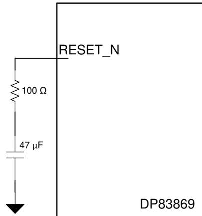
Figure 2. RESET\_N Circuit
