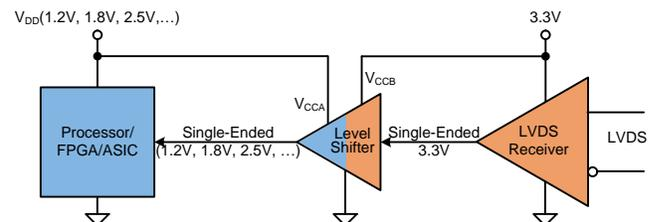
Figure 4. Using a Level-Shifter to Interface a 3.3-V LVDS Receiver to a Low-Voltage Device
