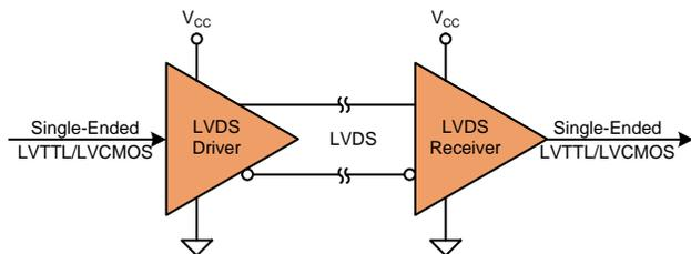
Figure 1. Operation of LVDS Drivers and Receivers
