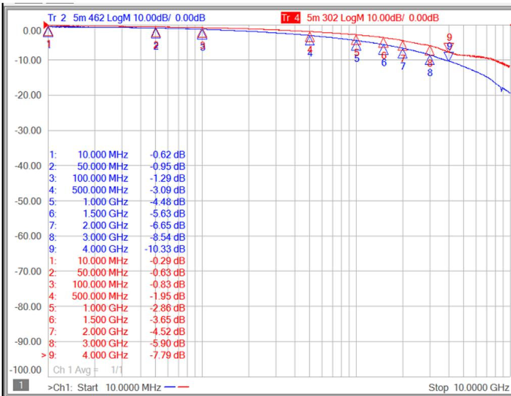
Figure 9. Insertion Loss for 5m Cables
