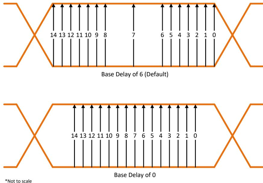
**Figure 4. Base Delay Effect on Strobe Positions**
