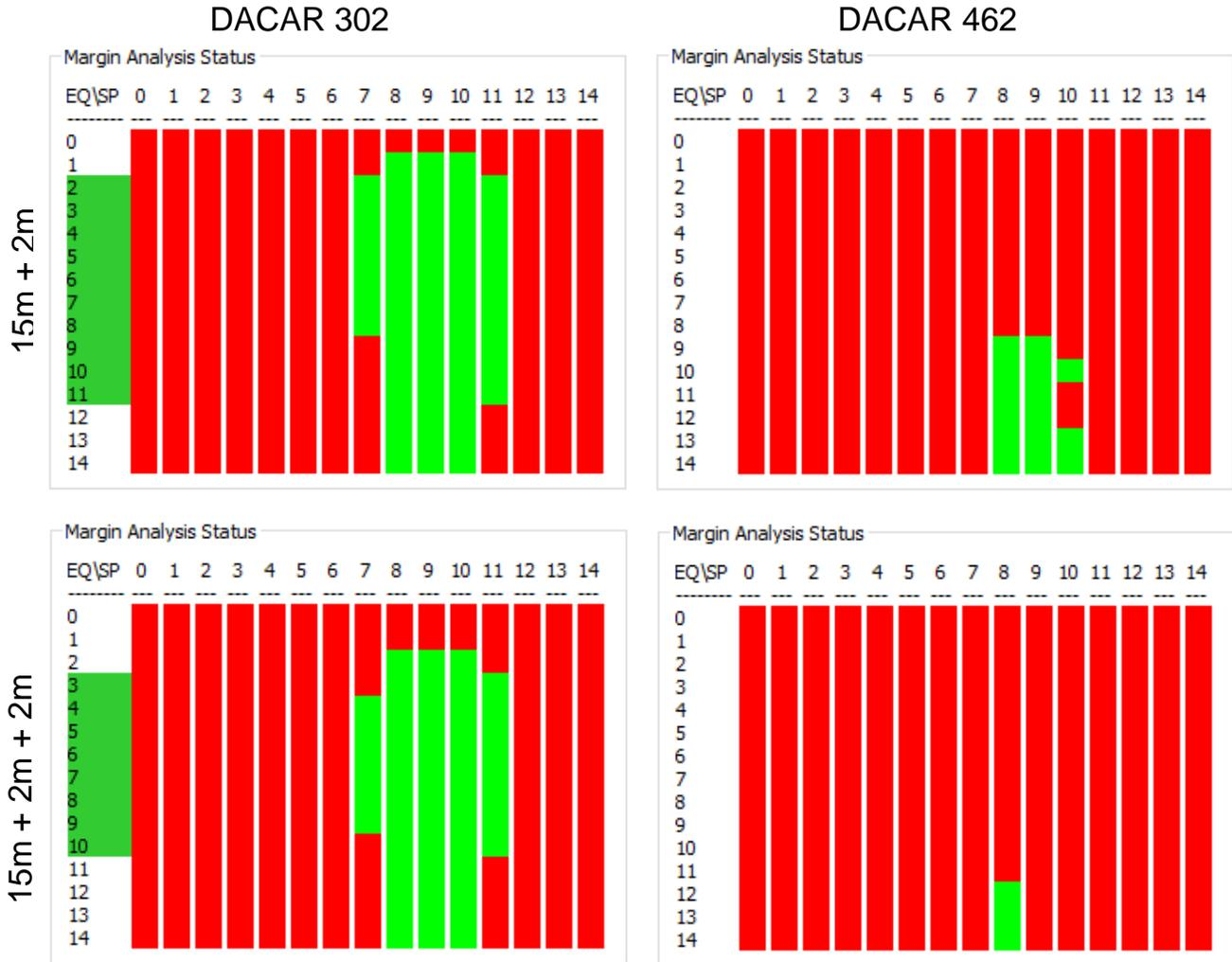
Figure 12. Margin Analysis Plots for Combined Cables With 0 Buffer Base Delay (1000-ms Dwell Time)
