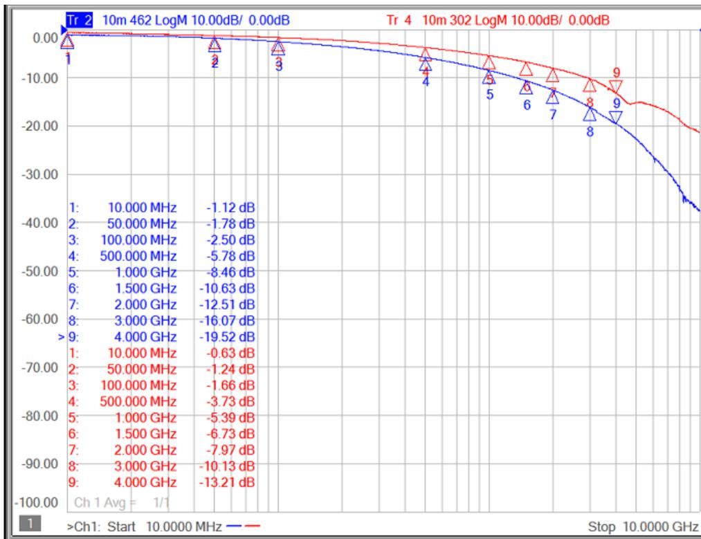
Figure 10. Insertion Loss for 10m Cables
