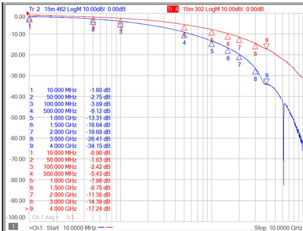
Figure 11. Insertion Loss for 15m Cables
