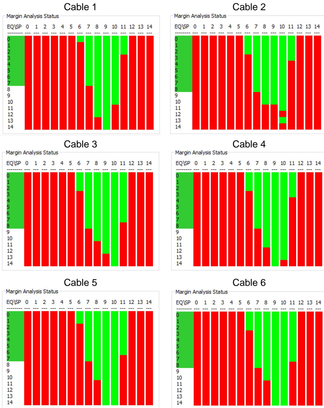
Figure 14. Margin Analysis Plots of Six Different 2m 462 Cables (Small Base Delay, 1000-ms Dwell Time)
