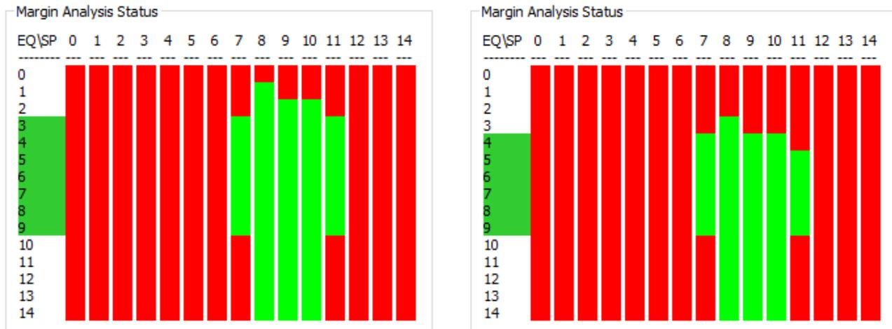
**Figure 13. Margin Analysis Plots for Combined Cable Types With 0 Buffer Base Delay (1000-ms Dwell Time)**
