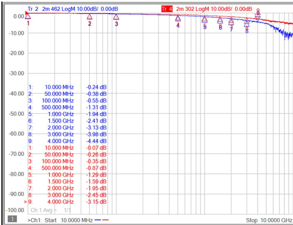
Figure 8. Insertion Loss for 2m Cables
