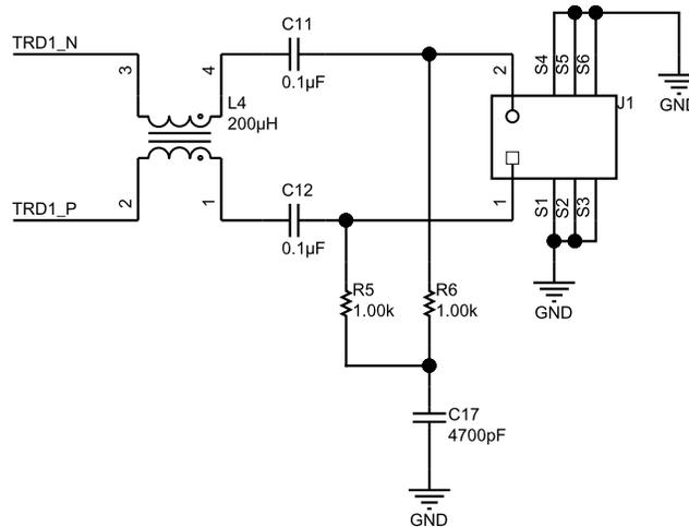
**Figure 10. PMA Schematic**
