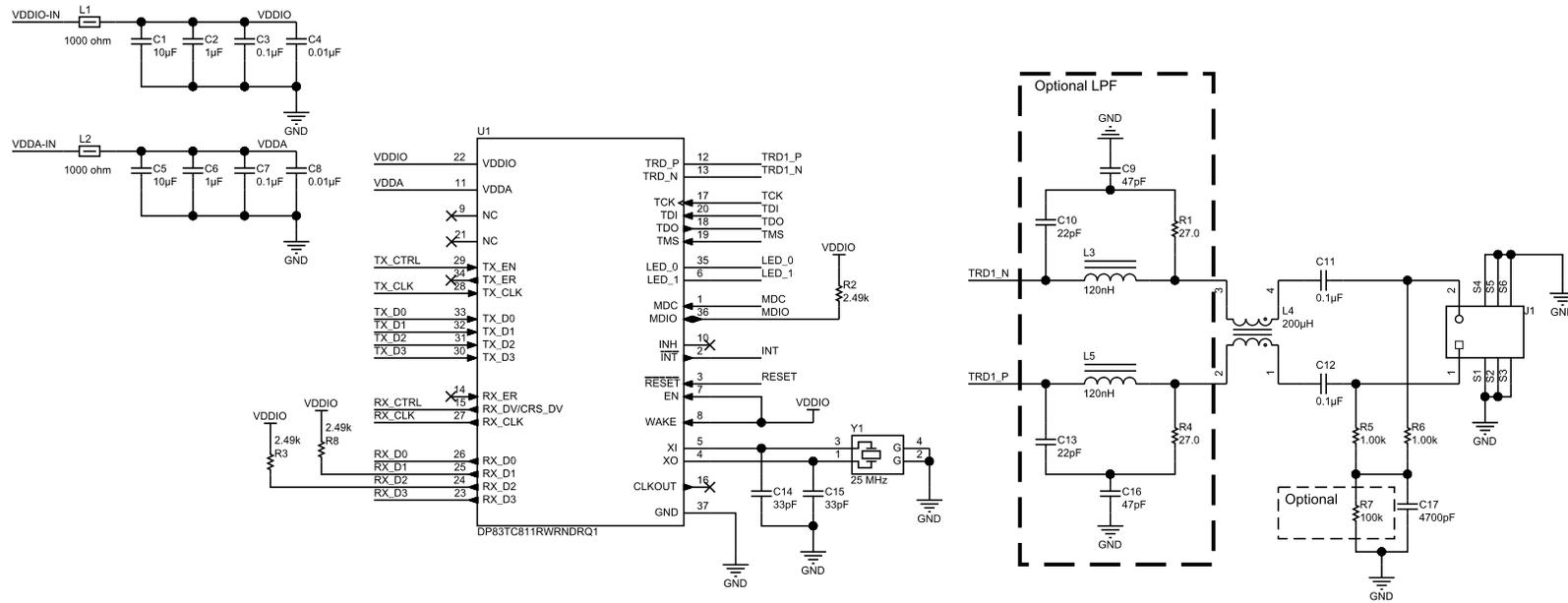
Figure 7. RGMII TX and RX Shift Schematic
