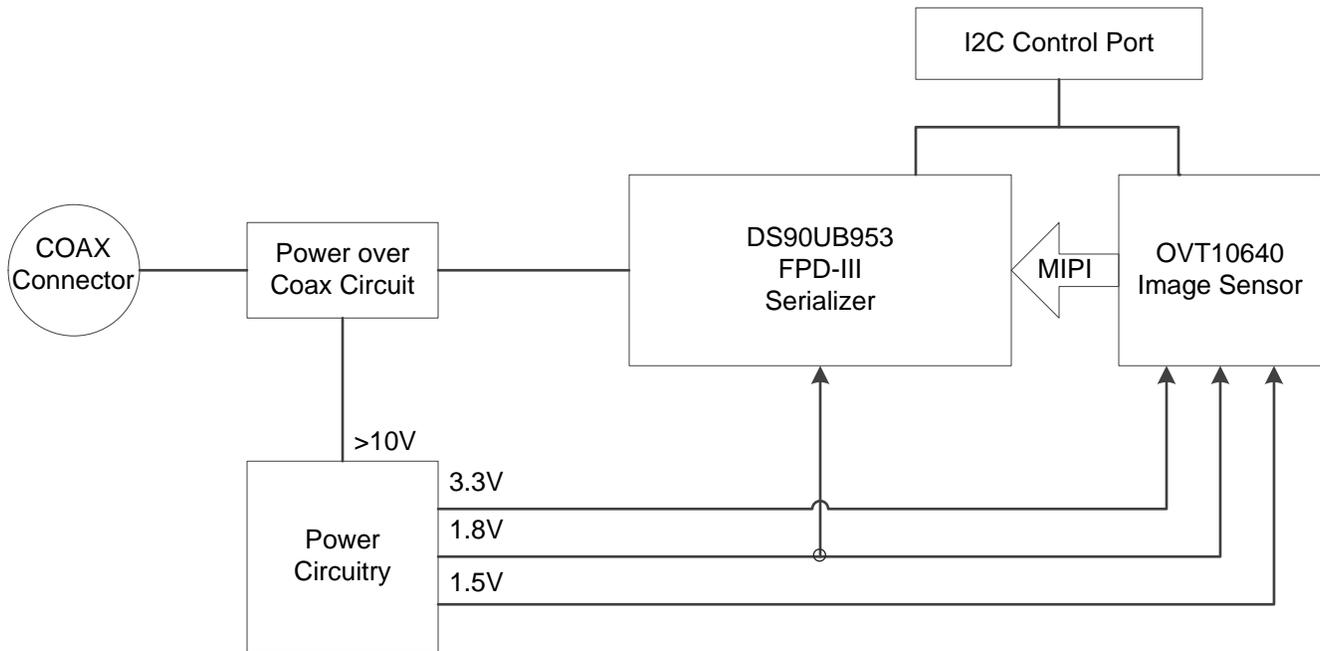
**Figure 1. DS90UB953-Q1 and Camera Block Diagram With Power-over-Coax (PoC)**
