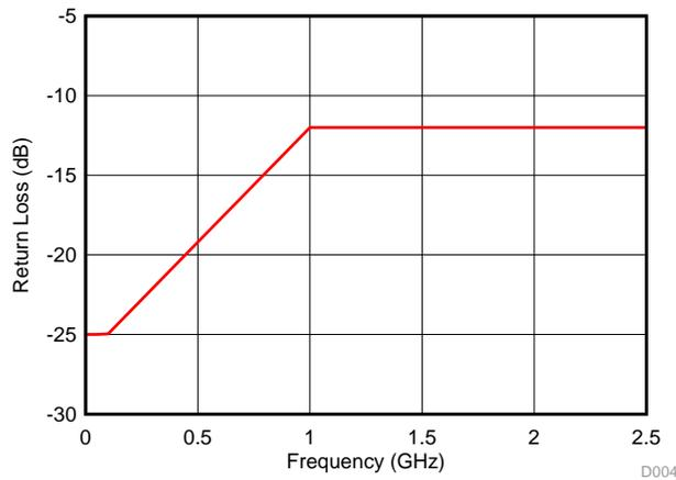
**Figure 3. Return Loss Specification Graph**
