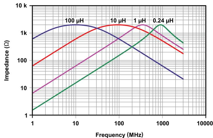
**Figure 4. Impedance Plot of Individual Inductors**
