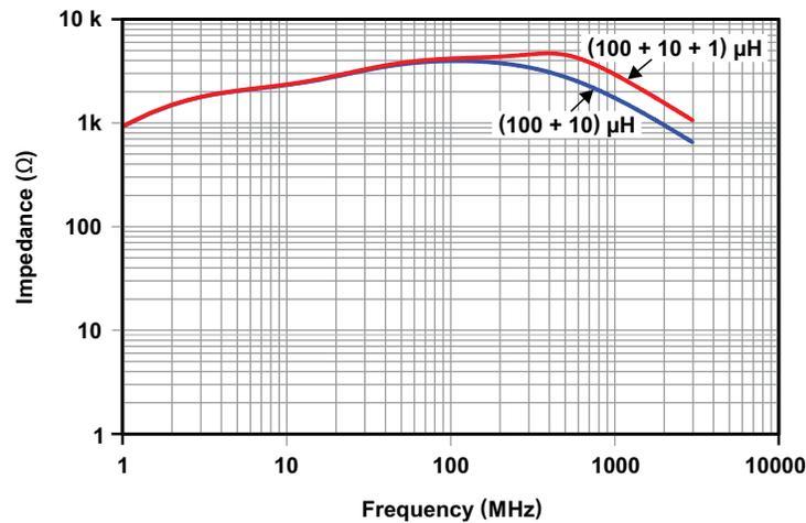
**Figure 5. Impedance Plot of a Wide-Bandwidth, Cascaded Inductor Network**
