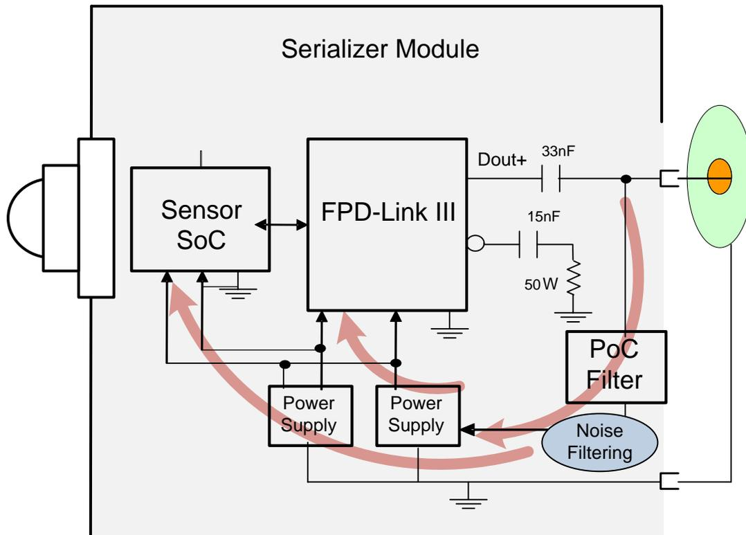
Figure 6. Sensor Current Flow
