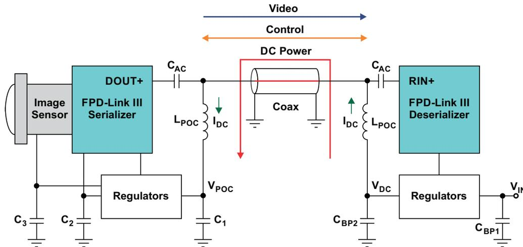
Figure 2. Block Diagram for Sharing Signal and DC Power on One Cable
