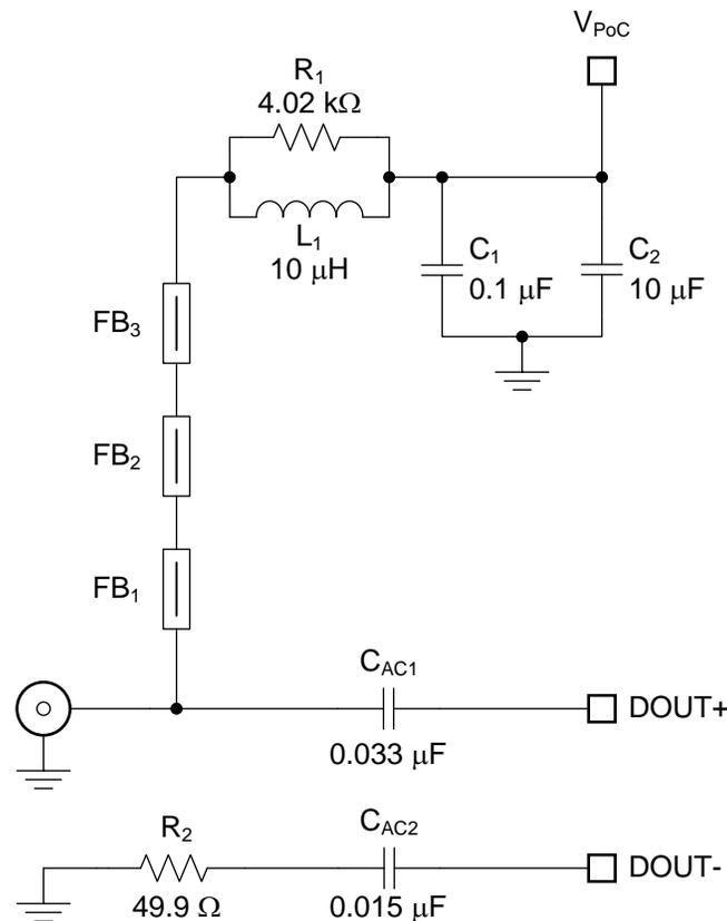
Figure 9. Typical PoC Network for a "4G" FPD-Link III
