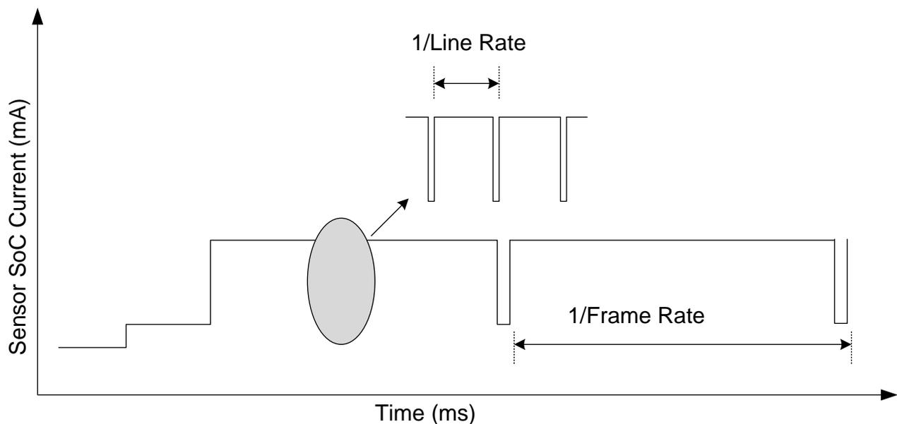
Figure 8. Sensor SoC Power Consumption vs. Time
