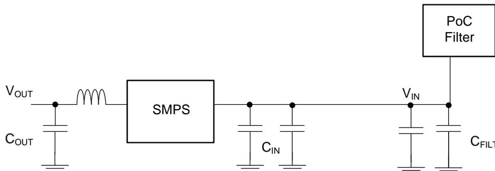
Figure 7. Switching Power Supply Filtering
