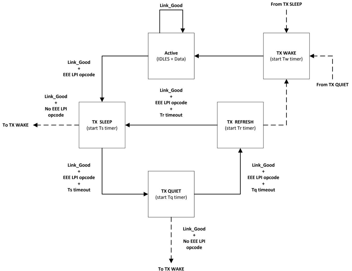
Figure 3. Transmit Path LPI State Diagram
