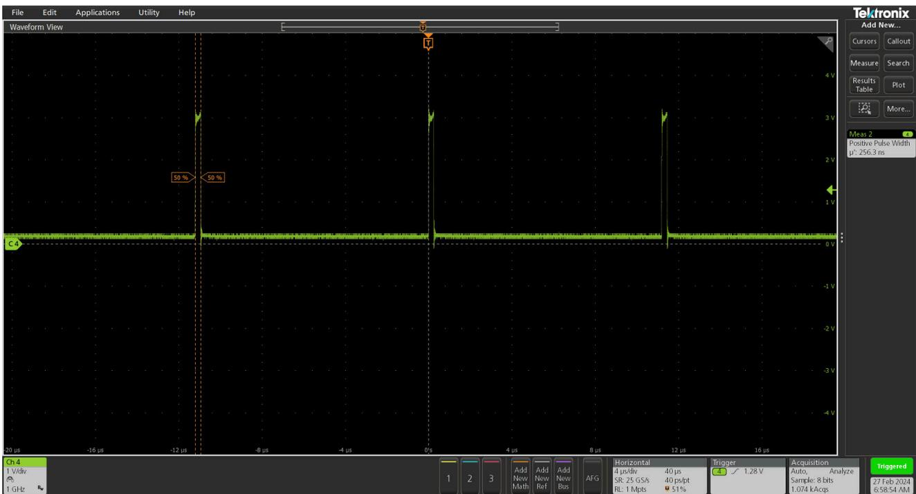
Figure 2-2. WoL Mechanism - 32 Clock Cycle
