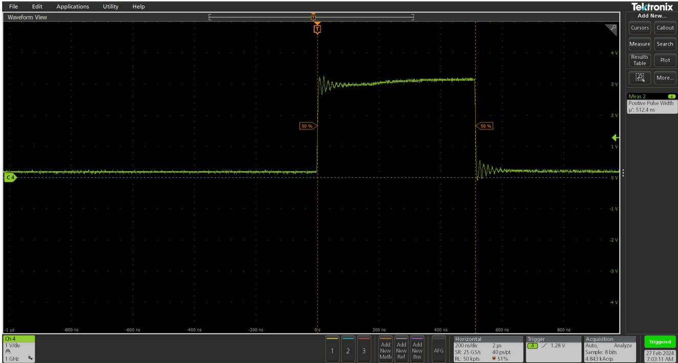
**Figure 2-3. WoL Mechanism - 64 Clock Cycle**
