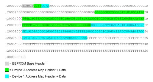
In the DS125DF111 hex file, the Base Header Bytes are 0x510010. From Table 2, this means:
