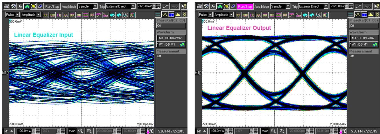
Figure 4. Waveforms Before and After a Linear Equalizer
