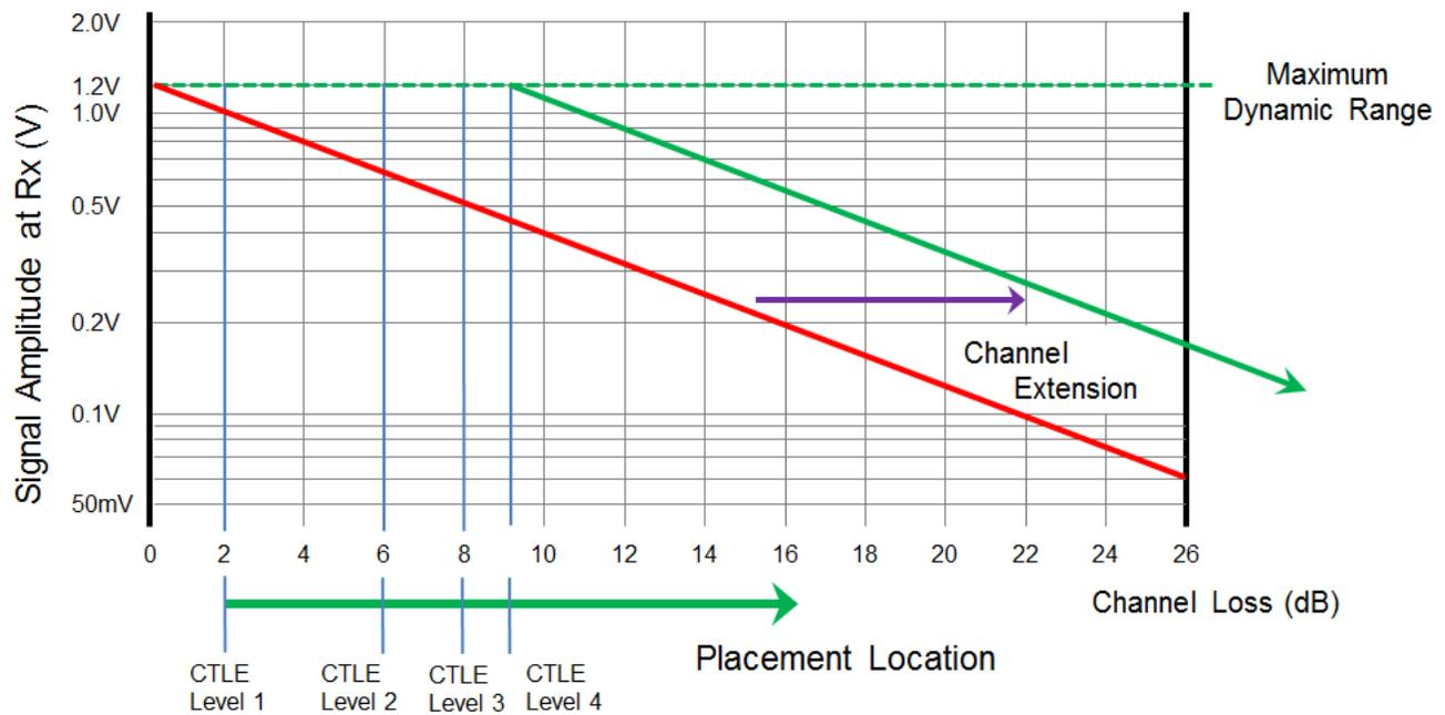
**Figure 5. Illustration of Channel Extension and DS125BR820 Placement**
