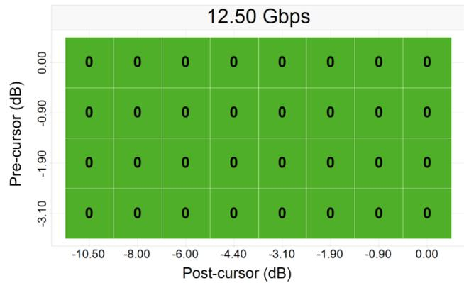
**Figure 33. 5" (-6.8 dB) Pre- and 25" (-27 dB) Post-channel with Redriver**
