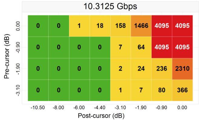
Figure 27. 15" (-14.5 dB) Pre- and 30" (-27.9 dB) Post-channel with Redriver
