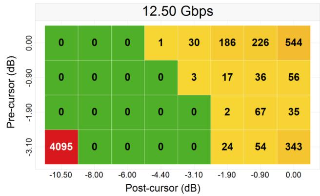
Figure 43. 10" (-11.9 dB) Pre- and 25" (-27 dB) Post-channel with Redriver
