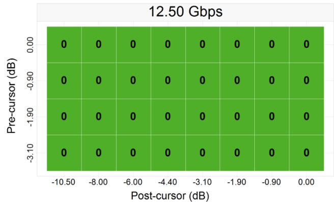
Figure 9. 5" (-6.8 dB) Pre- and 25" (-27 dB) Post-channel with Redriver
