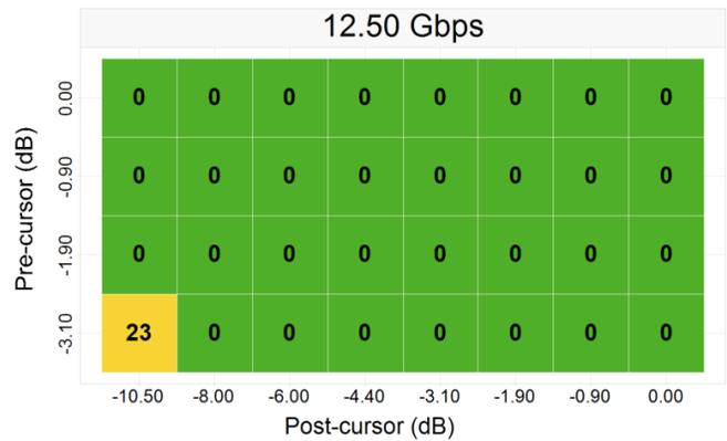
Figure 39. 25" (-27 dB) Pre- and 5" (-6.8 dB) Post-channel with Redriver
