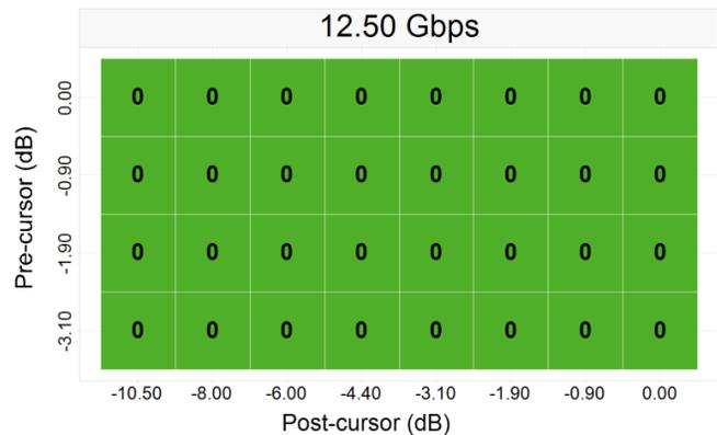
**Figure 35. 10" (-11.9 dB) Pre- and 20" (-22.1 dB) Post-channel with Redriver**
