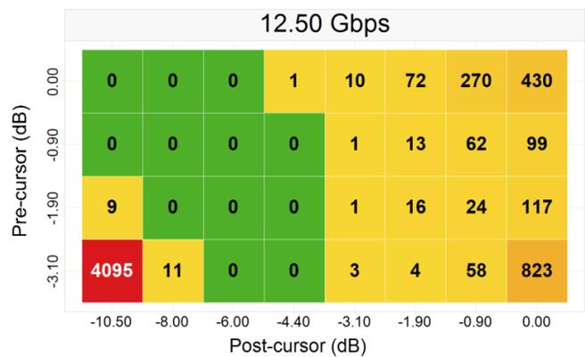
Figure 47. 30" (-32.9 dB) Pre- and 5" (-6.8 dB) Post-channel with Redriver
