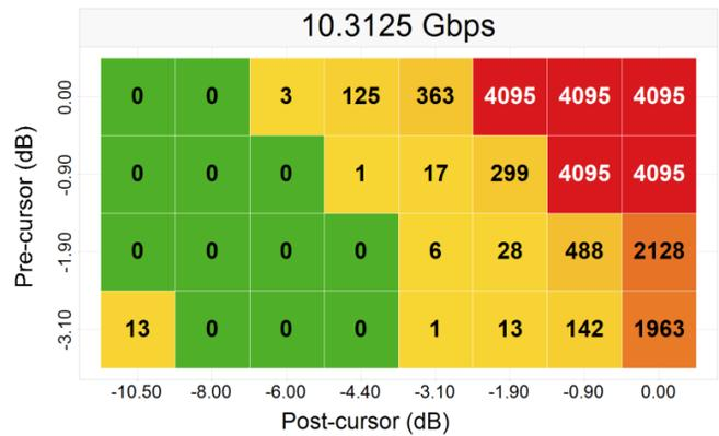
Figure 29. 30" (-27.9 dB) Pre- and 15" (-14.5 dB) Post-channel with Redriver
