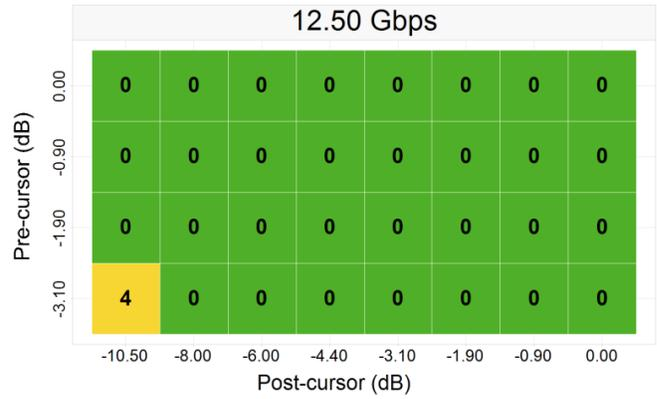
Figure 37. 20" (-22.1 dB) Pre- and 10" (-11.9 dB) Post-channel with Redriver
