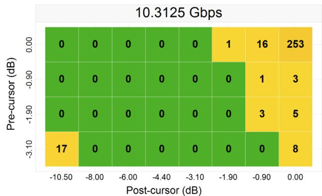
Figure 23. 35" (-31.9 dB) Pre- and 5" (-5.7 dB) Post-channel with Redriver
