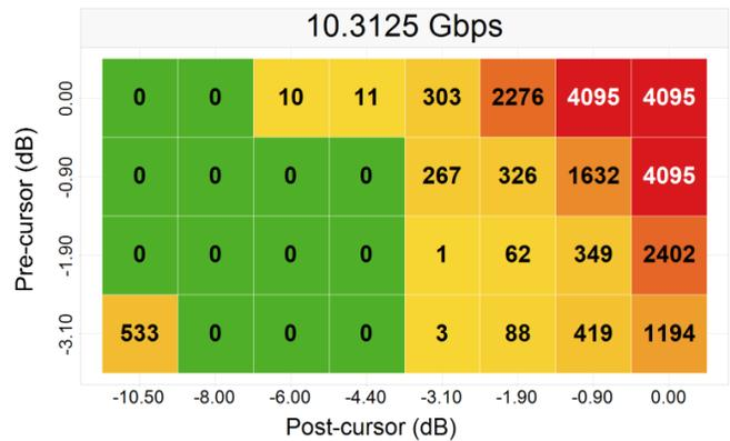
Figure 31. 40" (-35.3 dB) Pre- and 5" (-5.7 dB) Post-channel with Redriver
