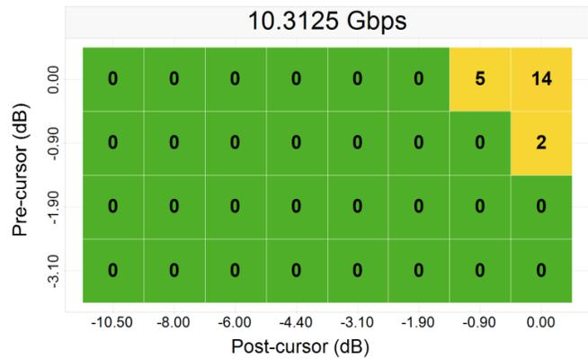
**Figure 17. 5" (-5.7 dB) Pre- and 35" (-31.9 dB) Post-channel with Redriver**
