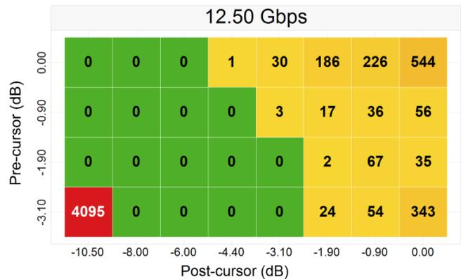
Figure 11. 10" (-11.9 dB) Pre- and 25" (-27 dB) Post-channel with Redriver
