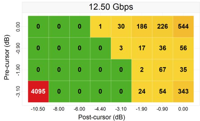
**Figure 15. 10" (-11.9 dB) Pre- and 25" (-27 dB) Post-channel with Redriver**
