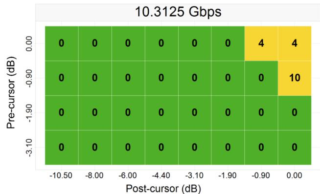
**Figure 19. 15" (-14.5 dB) Pre- and 25" (-22.9 dB) Post-channel with Redriver**
