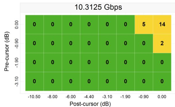
**Figure 5. 5" (-5.7 dB) Pre- and 35" (-31.9 dB) Post-channel with Redriver**
