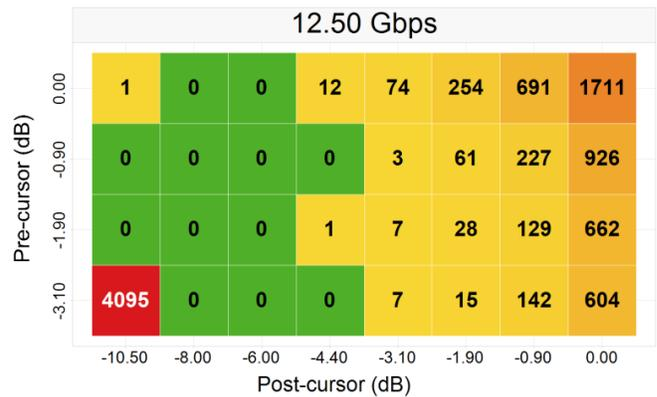
Figure 41. 5" (-6.8 dB) Pre- and 30" (-32.9 dB) Post-channel with Redriver
