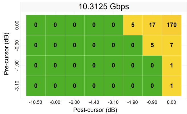
Figure 21. 25" (-22.9 dB) Pre- and 15" (-14.5 dB) Post-channel with Redriver
