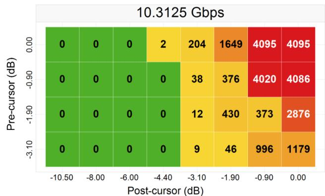
Figure 25. 5" (-5.7 dB) Pre- and 40" (-35.3 dB) Post-channel with Redriver
