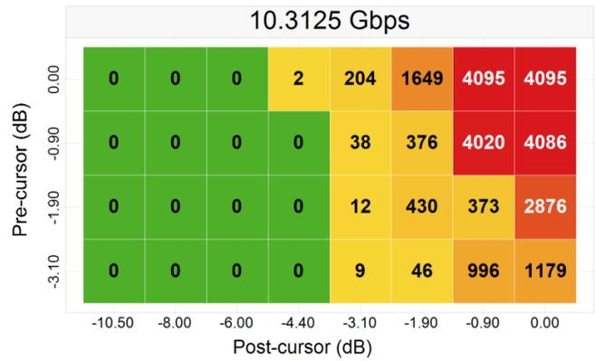
**Figure 13. 5" (-5.7 dB) Pre- and 40" (-35.3 dB) Post-channel with Redriver**
