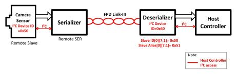
Figure 4. Communication with Remote slave/Camera attached to Remote SER
