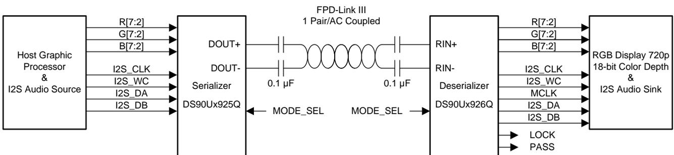
Figure 7. 4-Audio Channel Operation for DS90Ux925/926
