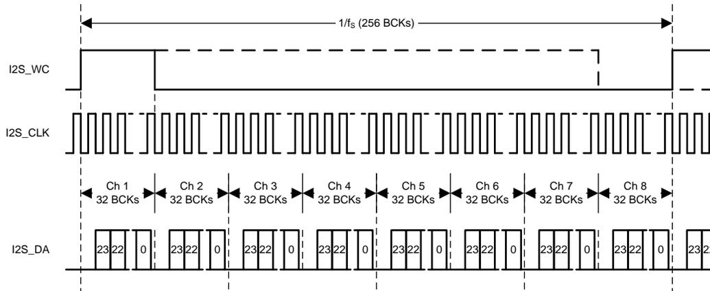
**Figure 3. TDM Example: 8 Audio Channels Multiplexed**
