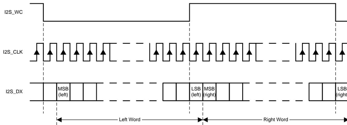
**Figure 2. I2S Frame timing diagram**
