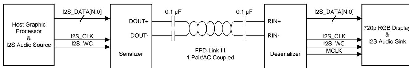
**Figure 1. Generic I2S Operation on SER/DES link**
