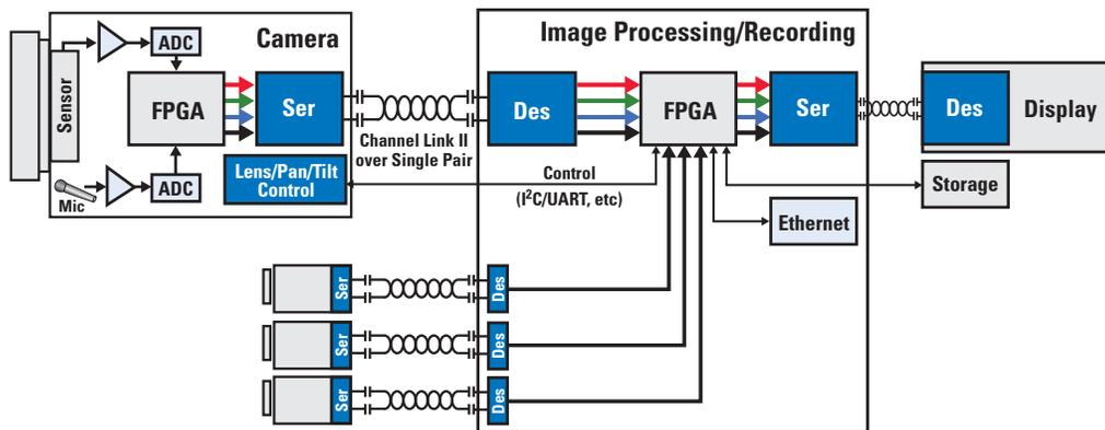
Figure 3-3. Example of a Security Camera System Block Diagram using Channel Link II Ser/Des
