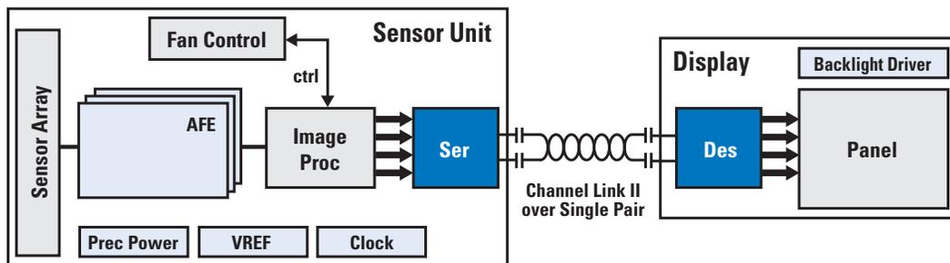
Figure 3-4. Example of a Medical Imaging System Block Diagram using Channel Link II Ser/Des
