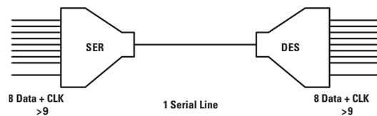
Figure 1-2. Ser/Des Devices reduce Wire Count
