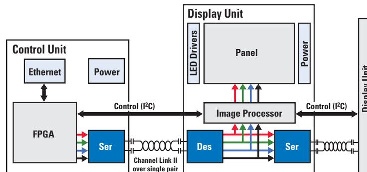
Figure 3-2. Example of a Display Signage Block Diagram using Channel Link II Ser/Des
