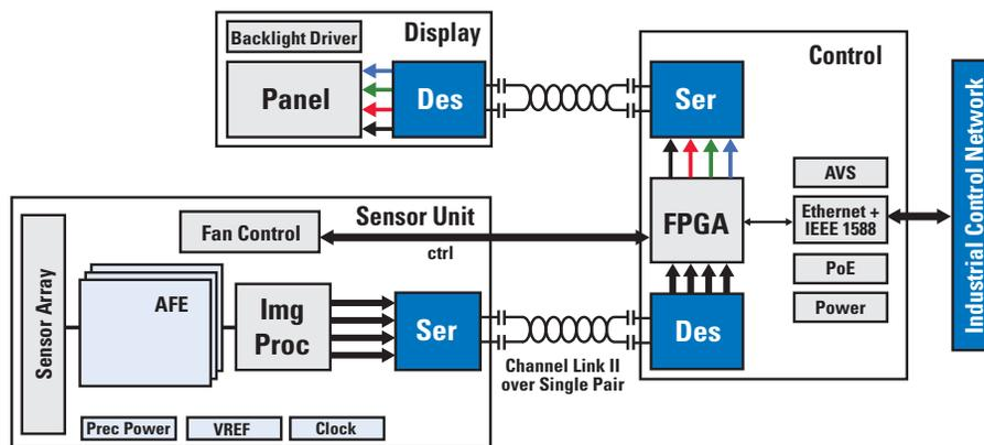
Figure 3-6. Example of a Factory Automation System Block Diagram with Channel Link II Ser/Des
