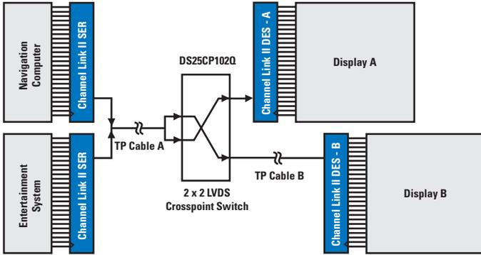
Figure 8-2. Example of a Video Application with Channel Link II and Crosspoint Switching
