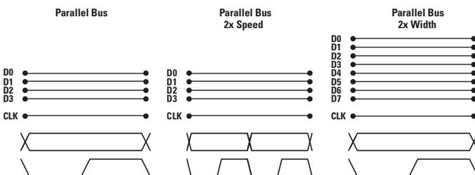
Figure 1-1. Increasing Bandwidth on a Parallel Point-to-Point Bus
