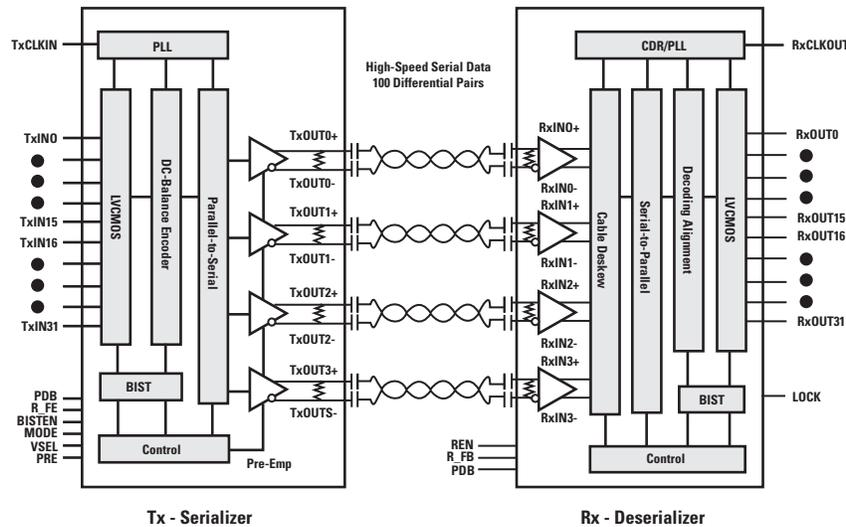
Figure 3-1. Example of a General-Purpose Channel Link II Ser/Des Application
