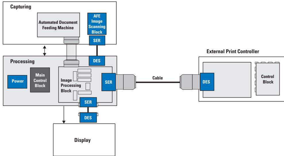
Figure 3-5. Example of a Multifunction Printer Block Diagram utilizing Channel Link II Ser/Des
