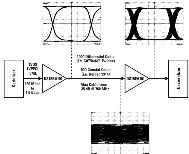
Figure 8-1. Example of a Cable Buffering/Extension Application
