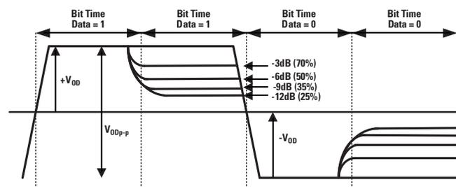
Figure 4-1. Serializer De-Emphasis Waveform (1100 Data Pattern)
