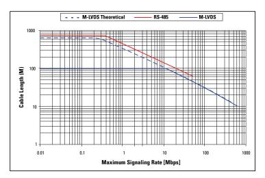
Figure 9-20. CAT-5e Length as a Function of Bit Rate for M-LVDS and RS-485 Point-to-Point Links
