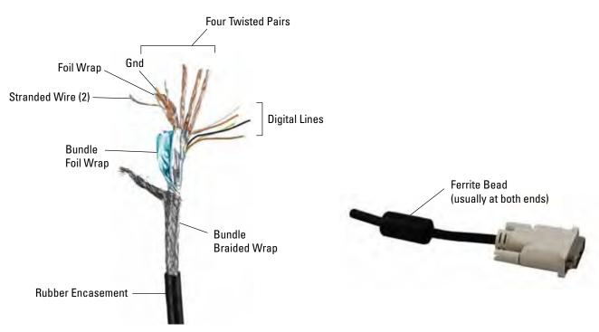
Figure 7-2. Stripped DVI Cable, Exposing Multiple Insulations
