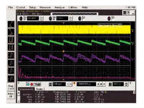
Figure 6-6. Example of Periodic Jitter
