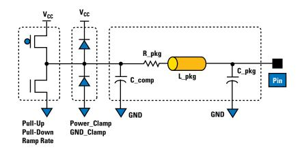
Figure 8-2. The IBIS 3-State Output Structure Model - The package characteristics and ESD structures are included and use the same notation as the input model
