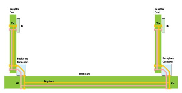
Figure 5-5. A Simplified Backplane Subsystem
