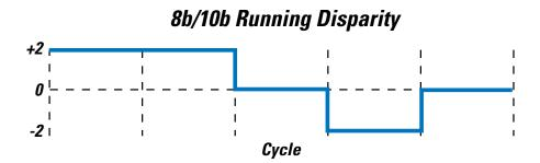
Figure 3-13. 8b/10b Running Disparity Example
