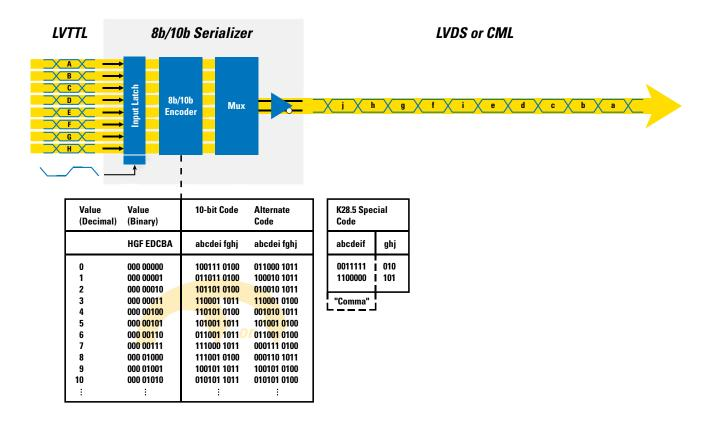
Figure 3-4. 8b/10b-Serializer Coding Example
