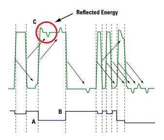
Figure 6-5. An Example of ISI-Pattern-Dependent Jitter and Reflections
