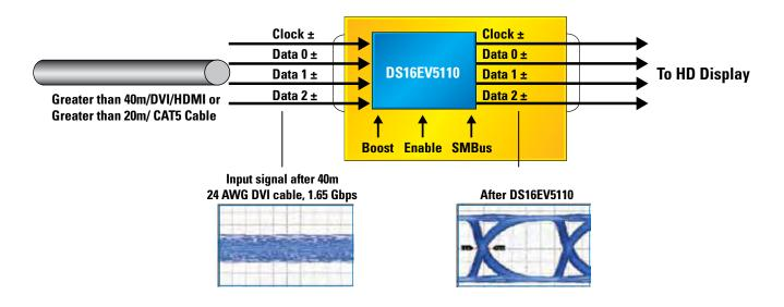
Figure 9-28. Using Signal-Conditioning ICs Extends Cable Performance
