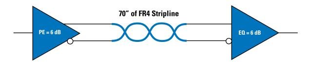
Figure 7-20. Output Pre-Emphasis Device Set to 6 dB PE Driving a 70" Trace into an Input Equalization Device Set to -6 dB EQ
