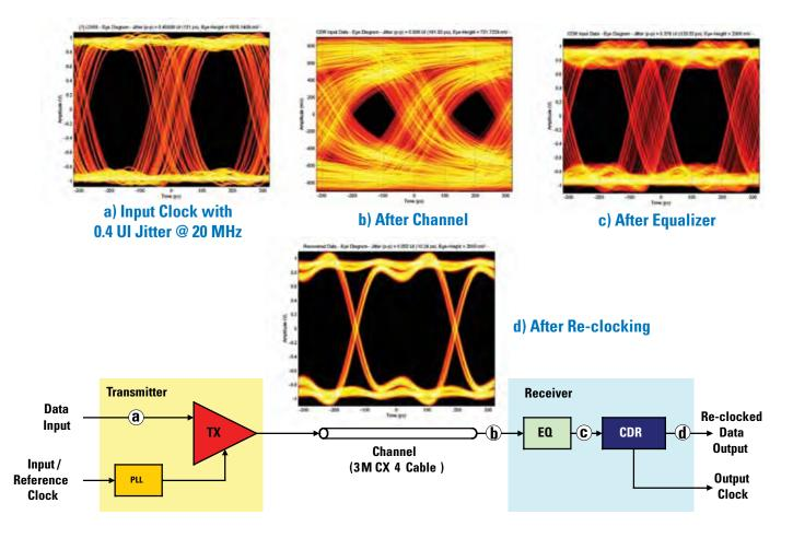
Figure 7-14. Recovered Signal Using Equalization and Re-clocking
