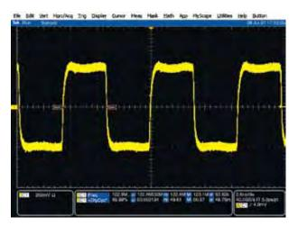
Figure 9-6. LMK03000 Clock-Conditioner Output
