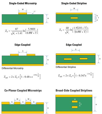
Figure 5-1. Controlled-Impedance Transmission Lines
