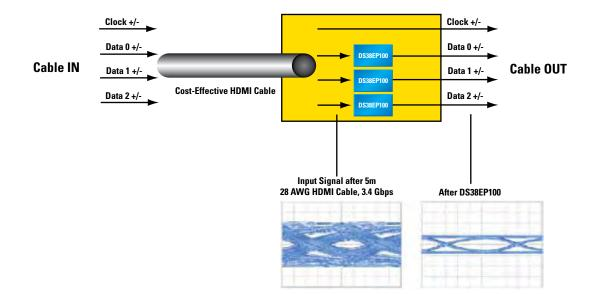
Figure 9-18. Power-Saver Equalization
