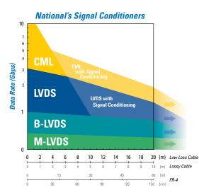
Figure 1-3. Typical Data Rates and Cable Drive Strength
