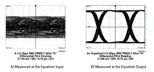
Figure 9-17. 2.5 Gbps NRZ Signal after 70" of FR-4 without Equalization (A) and with Equalization (B)
