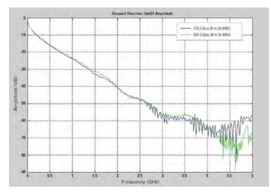
Figure 7-3. DVI Cable Loss vs. Wire Gauge
