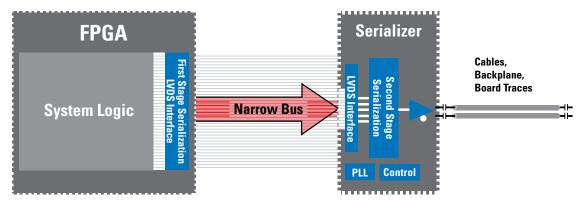
Figure 3-5. FPGA-Attach Serializer Optimizes the Analog-Intensive Functions
