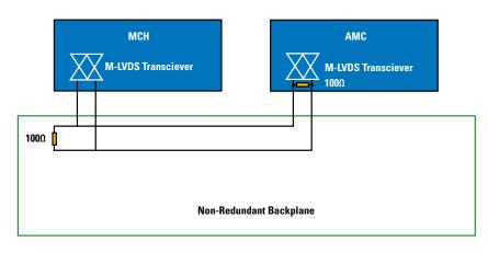
Figure 9-8. MicroTCA Non-Redundant Clock-Distribution Interface Example
