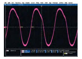
Figure 9-5. M-LVDS Clock Signal on a Fully-Loaded ATCA Backplane
