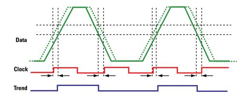
Figure 6-3. DCD Jitter Causes Timing Shifts
