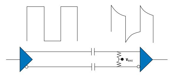
Figure 4-2. AC Coupling and Waveforms
