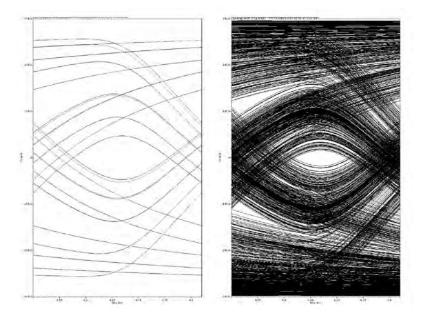
Figure 6-11. Comparison of a K28.5 Pattern (Left) with PRBS 31 Pattern (Right) after 41 Inches of FR4 Media. Plot Shows Degradation of Eye with Pattern Run Length.
