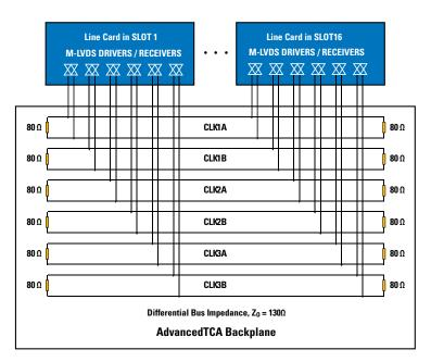
Figure 9-7. AdvancedTCA Clock-Distribution Interface Example
