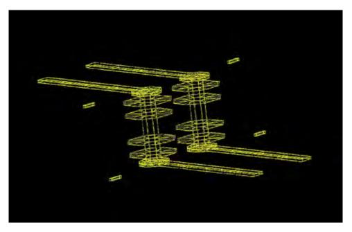
Figure 5-4. A 3-Dimensional Diagram of a Differential Via
