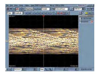
Figure 7-17. A 1.5 Gbps NRZ PRBS-7 after 200m of Belden 9914 Cable (No Correction); Scope: V:100 mV / DIV, H: 100 ps / DIV
