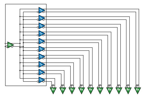
Figure 9-1. DS90LV110A 1-to-10 Fan-Out Buffer
