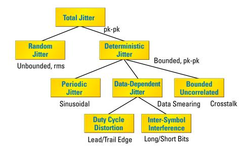
Figure 6-1. Jitter Components
