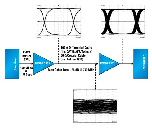
Figure 9-14. Typical Cable-Extender-Chipset Application
