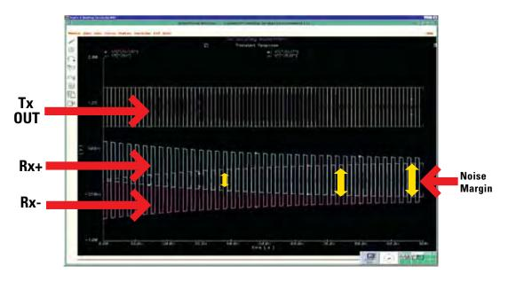
Figure 4-3. AC-Coupled Differential Pair at Startup
