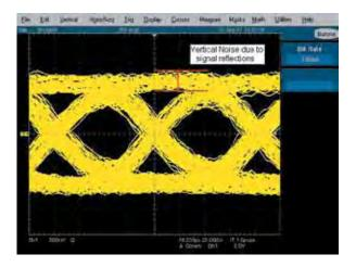
Increasing the data rate to 1 Gbps allows reflections from the driver and receiver to span almost 7 UI. The actual position of a signal at the receiver is being altered by any transitions during the previous seven data bits resulting in an eye diagram with a large DJ component.
