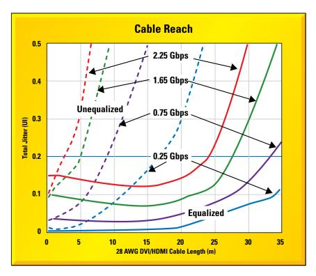
Figure 9-29. Different Cable Performance due to Correction-Enabled Signals
