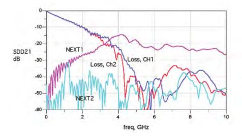
Figure 5-7. Transmission Characteristics of a 20-inch Backplane
