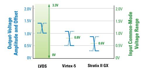
Figure 9-12. V<sub>0D</sub> versus Input Common-Mode Range of Various Differential Interfaces
