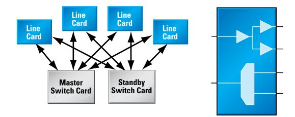
Figure 9-21. Simple Dual-Star Redundant Network
