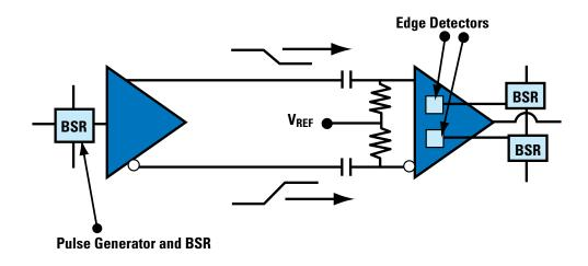
Figure 9-24. IEEE1149.6 Differential Test Standard
