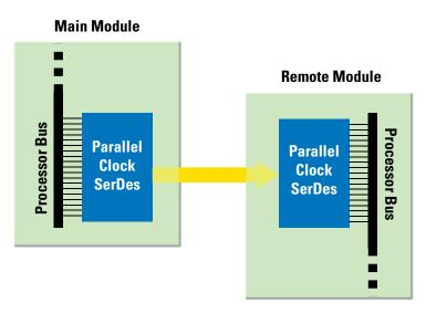
Figure 3-8. Unidirectional Rack-to-Rack Processor-Bus Extension
