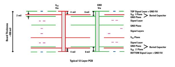
Figure 5-8. Low-Inductance, High-Capacitance Power Connection
