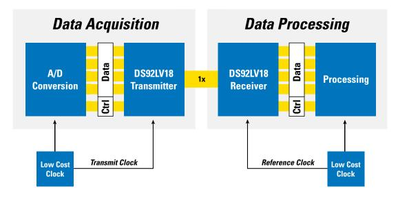
Figure 3-9. Signal-Processing System Implementation Based on DS92LV18 SerDes
