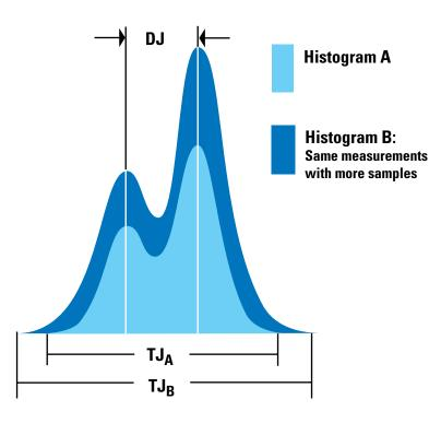
Figure 6-2. Total Jitter Histogram
