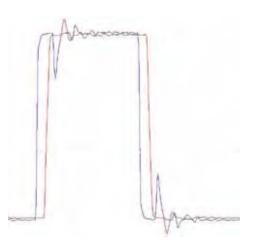
At 50 MHz, the simulation waveform shows reflections at the driver and receiver due to excess I/O capacitance, even with the transmission line properly terminated. These reflections will cause significant Inter-Symbol Interference (ISI) as the data rate is increased.
