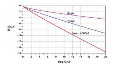
Figure 5-2. 10-Inch Microstrips Implemented with Different Board Materials
