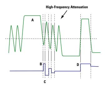
Figure 6-4. An Example of ISI-Pattern-Dependent Jitter and Reflections
