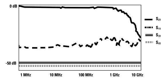
Figure 8-6. An Example of a Hypothetical Network with Stimulus Introduced at Node 1
