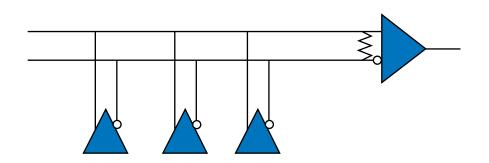
Figure 4-12. Example of Wired-Or Circuit
