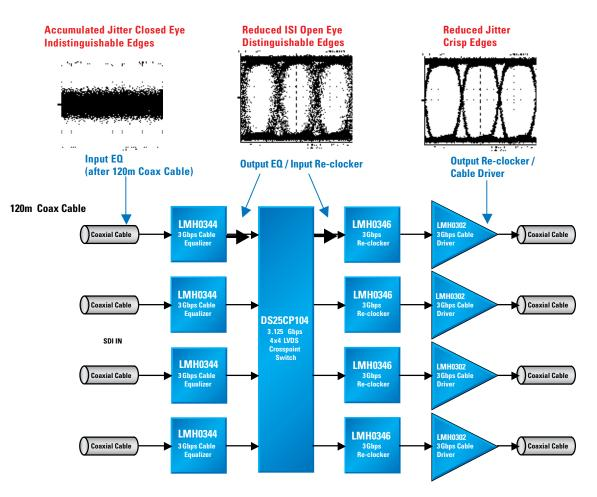
Figure 9-13. Simplified 3 Gbps Serial-Digital-Interface Video Router
