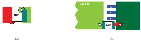
Figures 5-8a and 5-8b. Typical Decoupling Capacitor Layouts
