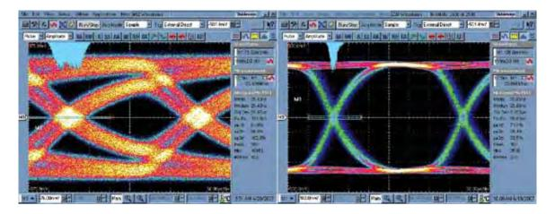
Figure 7-16. 3.125 Gbps Signal Going Through 28" of Differential FR4 Stripline on NRZ PRBS-7 Before (Left) Then After Equalizer Device (Right) (V: 125 mV / div., H: 50 ps / div.)
