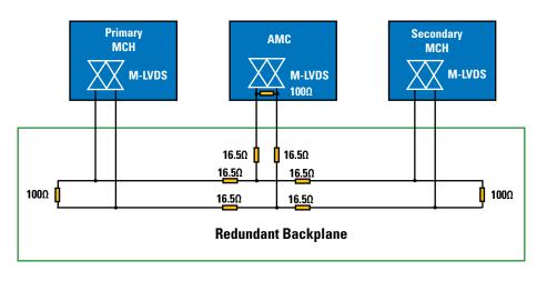
Figure 9-9. MicroTCA Redundant Clock-Distribution Interface Example
