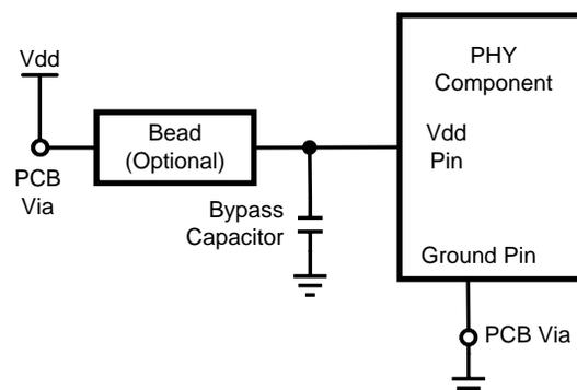
**Figure 4. Bypassing and Isolating Power and Ground Pins**
