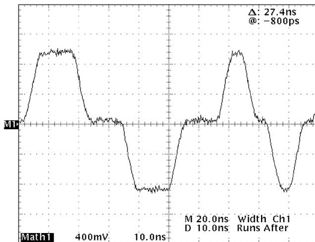
Figure 2. 100Mb Waveform
