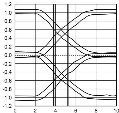
Figure 11. 100 Mb/s Jitter with 33 nf Blocking Capacitors
