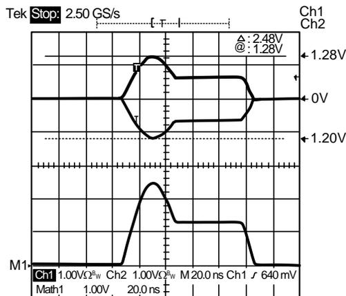
Figure 2. Sample Link Pulse waveform
