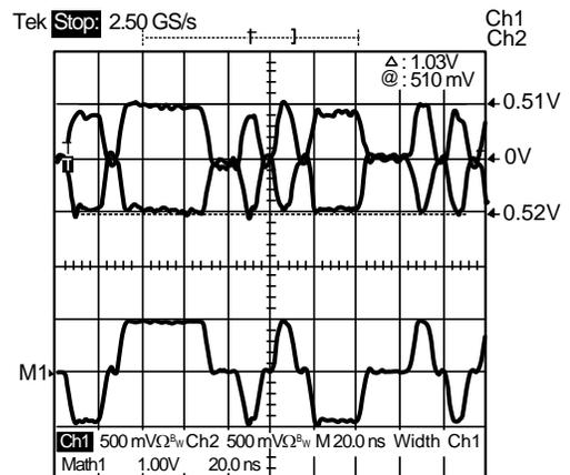
Figure 3. Sample 100 Mb/s Waveform (MLT-3)
