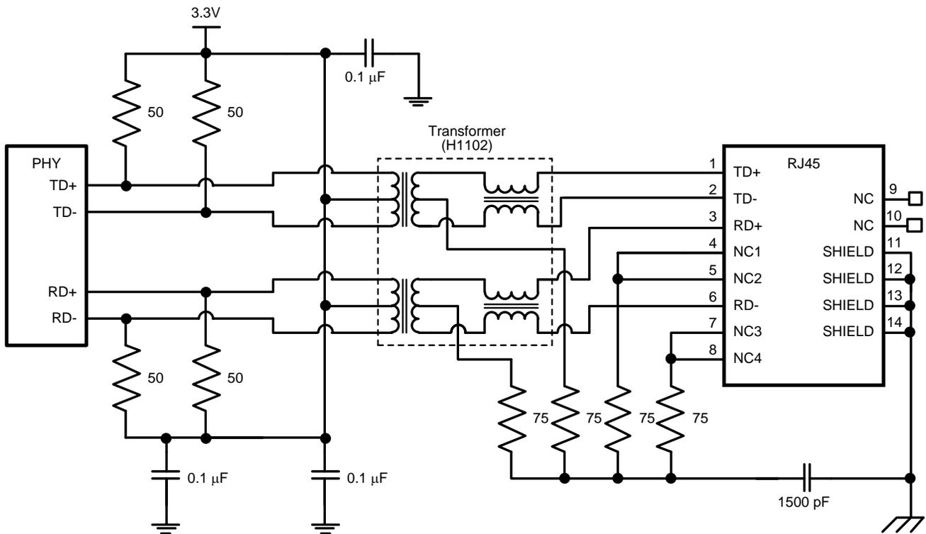
Figure 1. Typical 10/100 Mb/s Twisted Pair Interface
