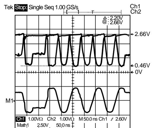
Figure 9. Sample 10 Mb/s Waveform With No Transformer
