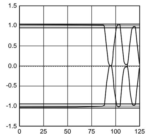
Figure 14. 100 Mb/s Vod with 33 nf Blocking Capacitors
