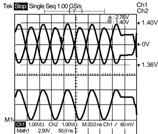
**Figure 4. Sample 10 Mb/s Waveform**
