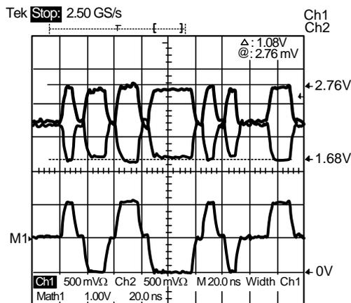
Figure 8. Sample 100 Mb/s Waveform With No Transformer
