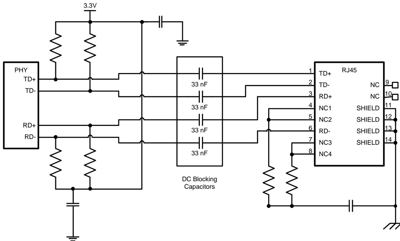
Figure 5. Transformerless Configuration
