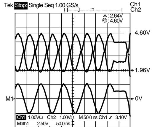
Figure 7. Sample 10 Mb/s Waveform
