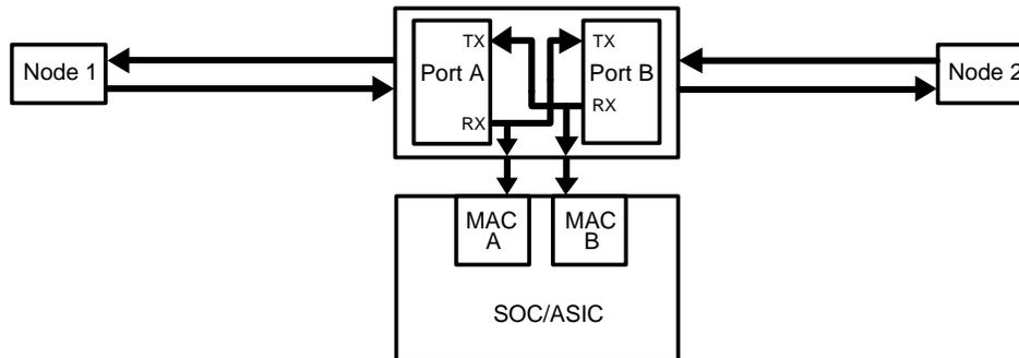
**Figure 8. Ethernet Snoop Device**
