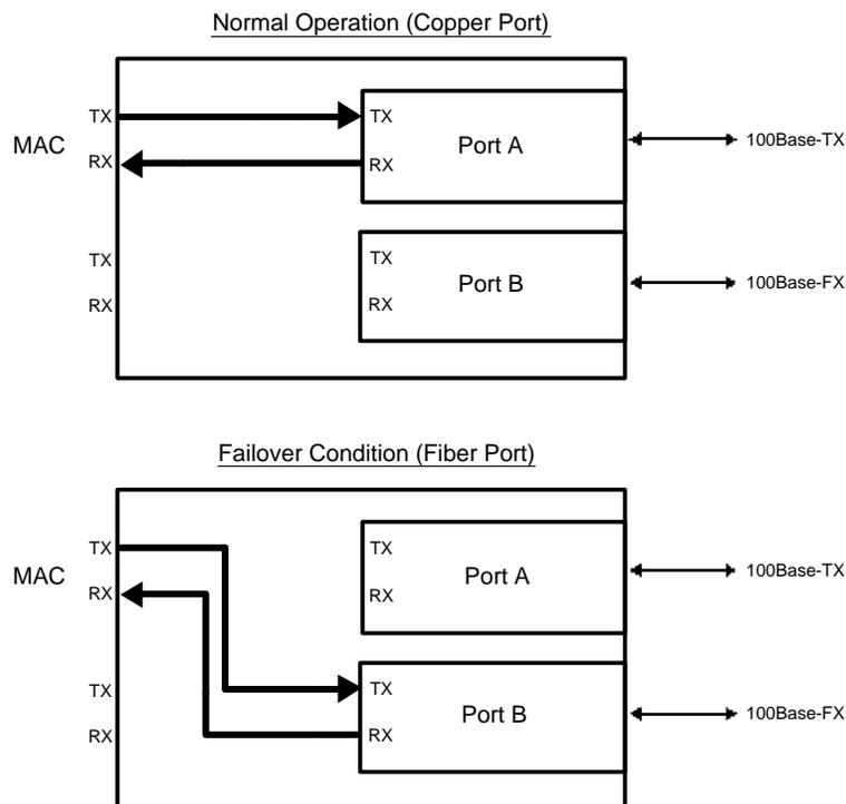
**Figure 5. Single with Dedicated Copper and Fiber Ports**
