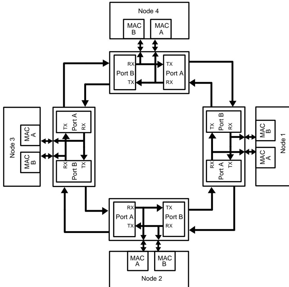
Figure 9. Ethernet Ring Example With 4 Nodes
