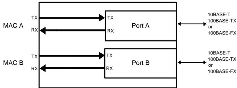
Figure 2. Normal Port Mapping
