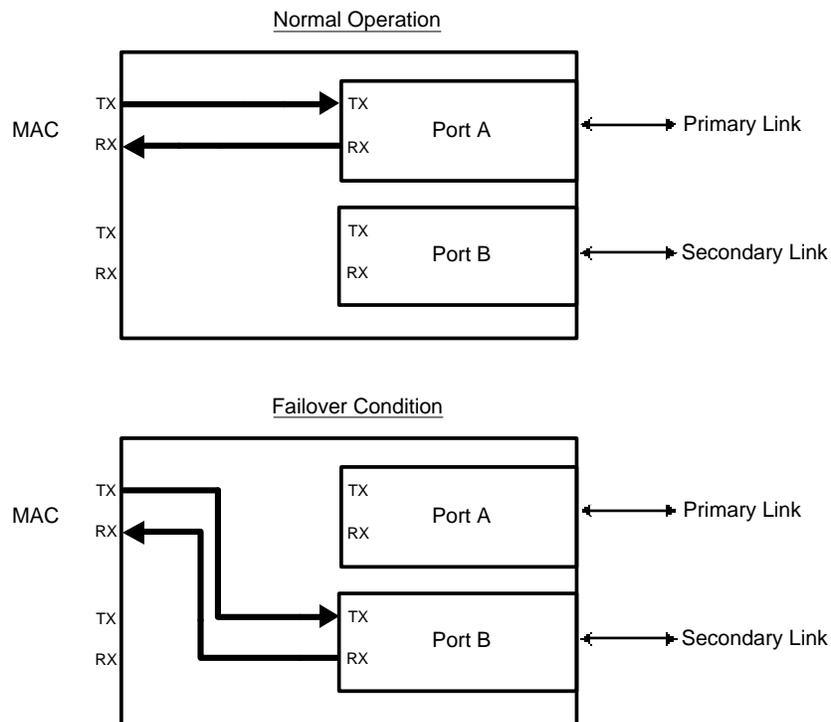
**Figure 4. Software-Assisted Failover**
