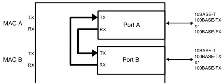
**Figure 20. Extender/Media Converter (Programmed with no RX monitoring)**
