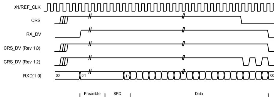
Figure 2. CRS\_DV Generation
