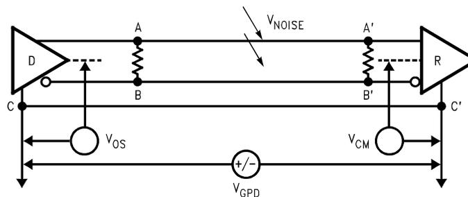
The common-mode voltage,  $V_{CM}$ , is the average of the voltages at a driver's two outputs or a receiver's two inputs. You measure all voltages with respect to the driver's or receiver's common terminal.
