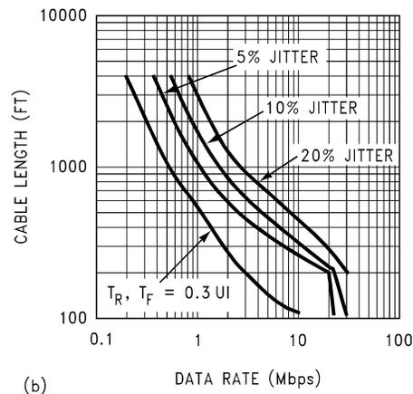
As you increase the cable length, the maximum data rate decreases. The more jitter you can accept, the greater is the allowable data rate for a given length of cable.
