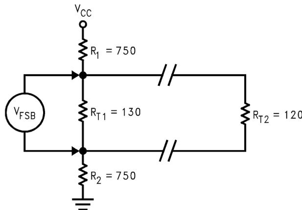
Unless you do something to keep the situation from occurring, when no driver is driving the bus, the receivers cannot determine the bus state. Fail-safe biasing is a bus-termination method, which ensures that, even when no driver is active, a differential voltage large enough to unambiguously determine the bus state appears at the receiver inputs.
