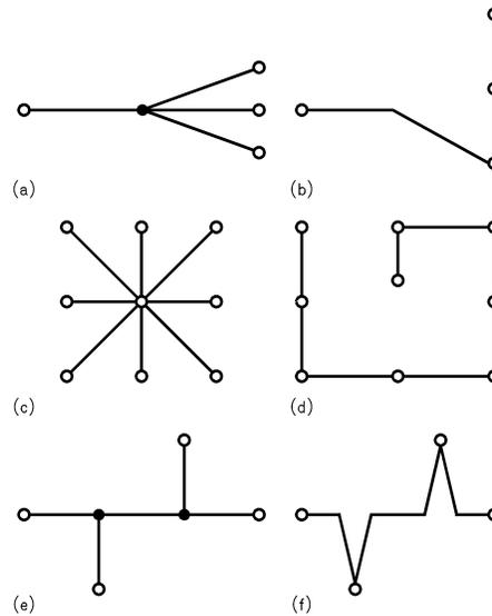
Although you can make RS-485 buses with all of these configurations work, you should avoid the ones in (a), (c), and (e). Those in (b), (d), and (f), offer superior transmission-line performance.
