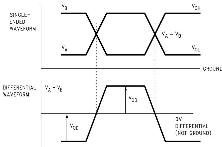
Although the voltages on the bus's two conductors vary symmetrically about a value that is halfway between the driver's Low and High output-state values, the differential voltage between the conductors varies about zero. In addition, the differential voltage swing is double the swing on either of the bus conductors.
