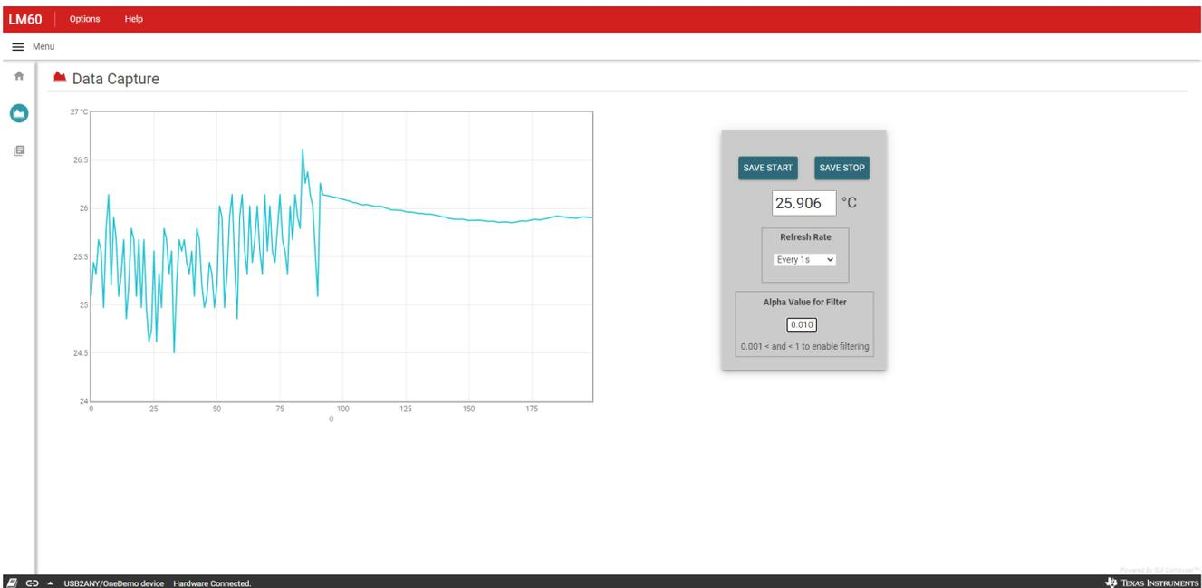
Figure 4-3. Data Capture After Filter Implemented
