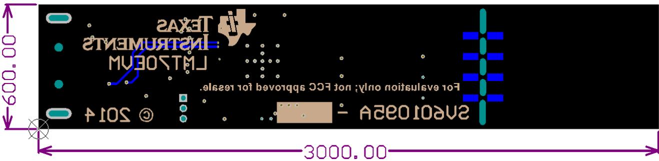
Figure 6-6. Bottom Assembly Layer
