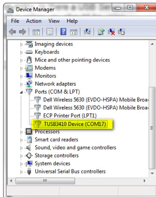
**Figure 3. Device Manager with COM Port Name**
