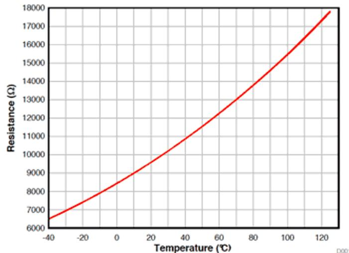
**Figure 3-2. TMP61 R-T Relationship Diagram**
