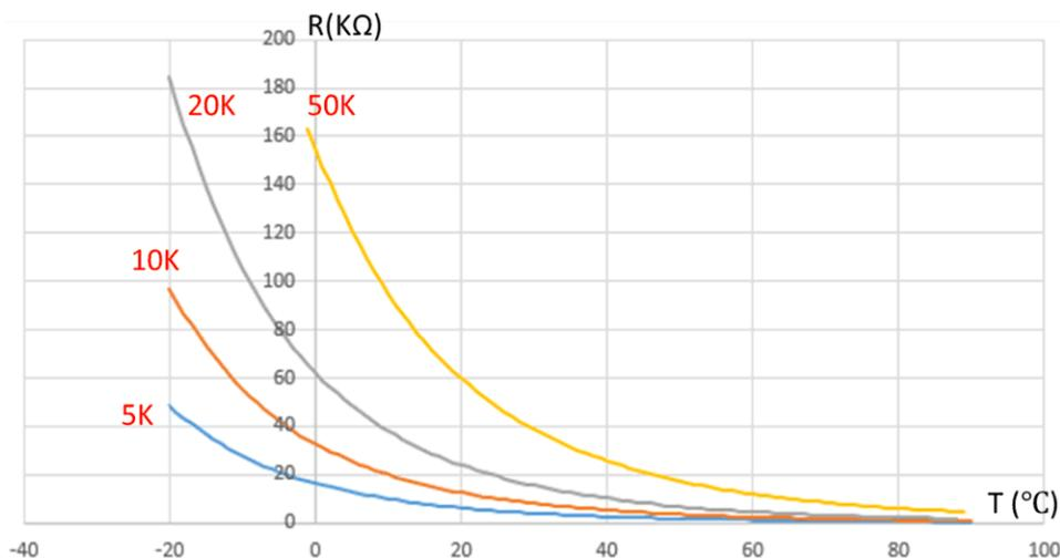
**Figure 2-1. Diagram of NTC R-T Relationship With Different Resistance Values**
