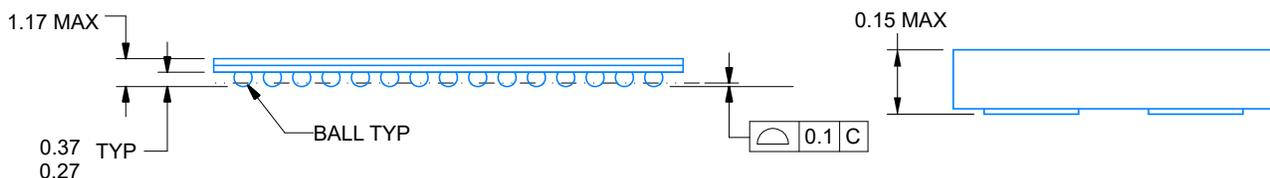
Figure 4-5. TMP114, TMP144, and IWR6843 Vertical Dimensions
