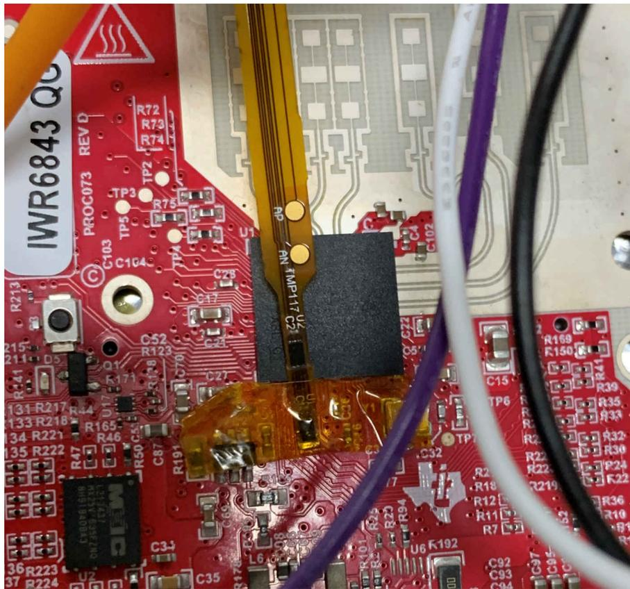
**Figure 4-8. TMP114 and TMP117 Temperature Sensor Testing Setup**
