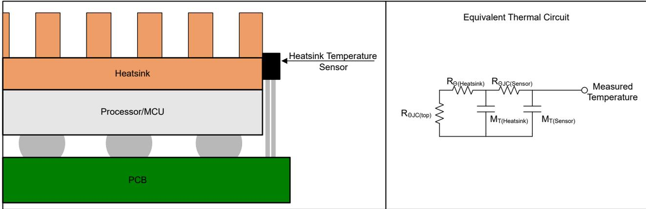
**Figure 2-1. Equivalent Thermal Circuit for Heat Sink Temperature Sensing**
