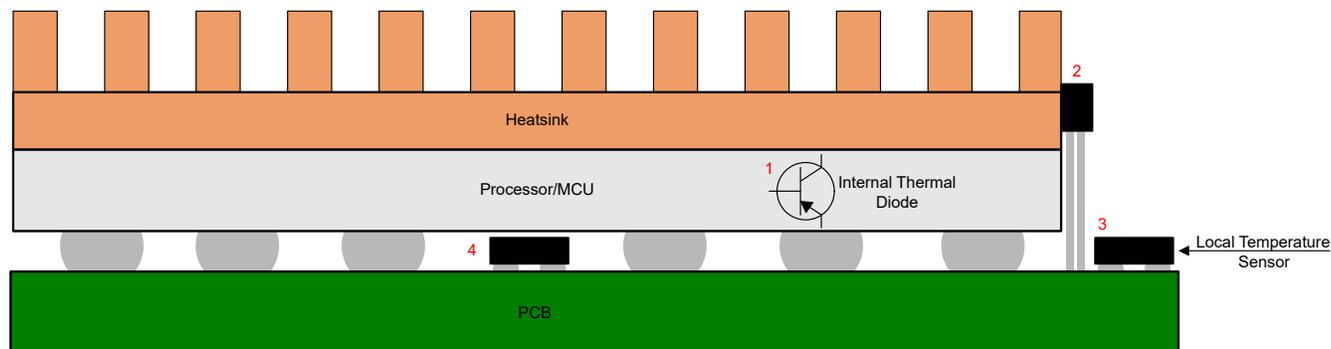
**Figure 1-1. SMT Processor Temperature Measurement Options**
