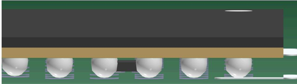
Figure 4-3. Board Rendering of TMP114 Temperature Sensor Underneath IWR6843 Sensor
