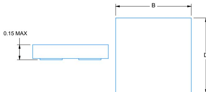
Figure 4-2. TMP144 and TMP144 YMT Package Drawing
