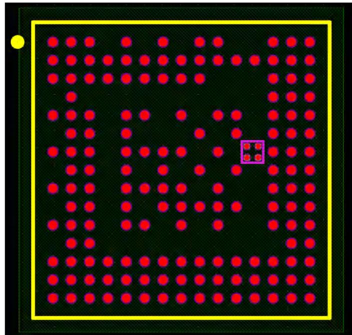
Figure 4-4. IWR6843 and TMP114 Footprints Rendered in PCB Editor
