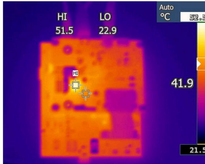
Figure 4-1. Thermal Capture of AWR2243BOOST Under Moderate Load
