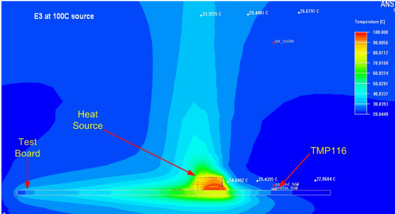
**Figure 3-1. Thermal Simulation of TMP116 near 100C Heat Source**
