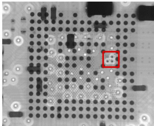
Figure 4-7. Xray Image of IWR6843 with TMP114 Temperature Sensor Underneath
