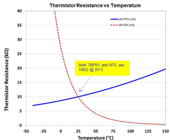
**Figure 1. Resistance vs Temperature of PTC vs NTC**
