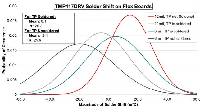
**Figure 3. Solder Shift on 12-mil and 6-mil Flex Boards When Compared to Readings Within an IC Socket.**
