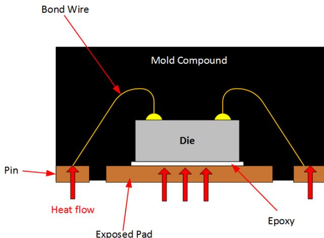
Figure 1. Cross Section of WSON (TMP117DRV) Package Showing Heat Transfer
