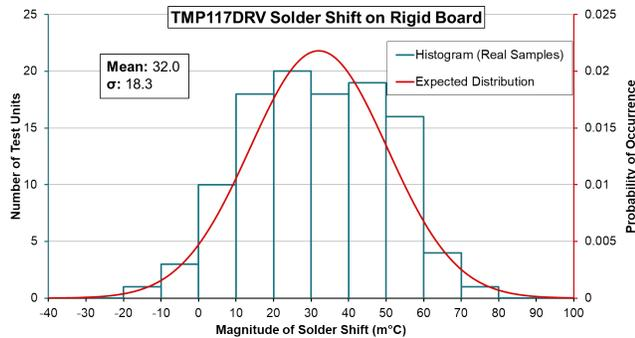
**Figure 2. Test Results for Soldering TMP117DRV to a Rigid Board. The Magnitude of Solder Shift was Around 32m°C on Average.**
