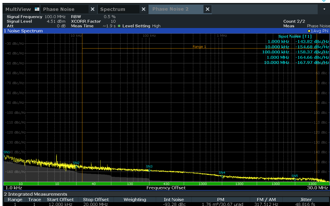
Figure 4-2. SMA100B 100MHz Input to LMK3H2108EVM for Buffer Mode Measurement
