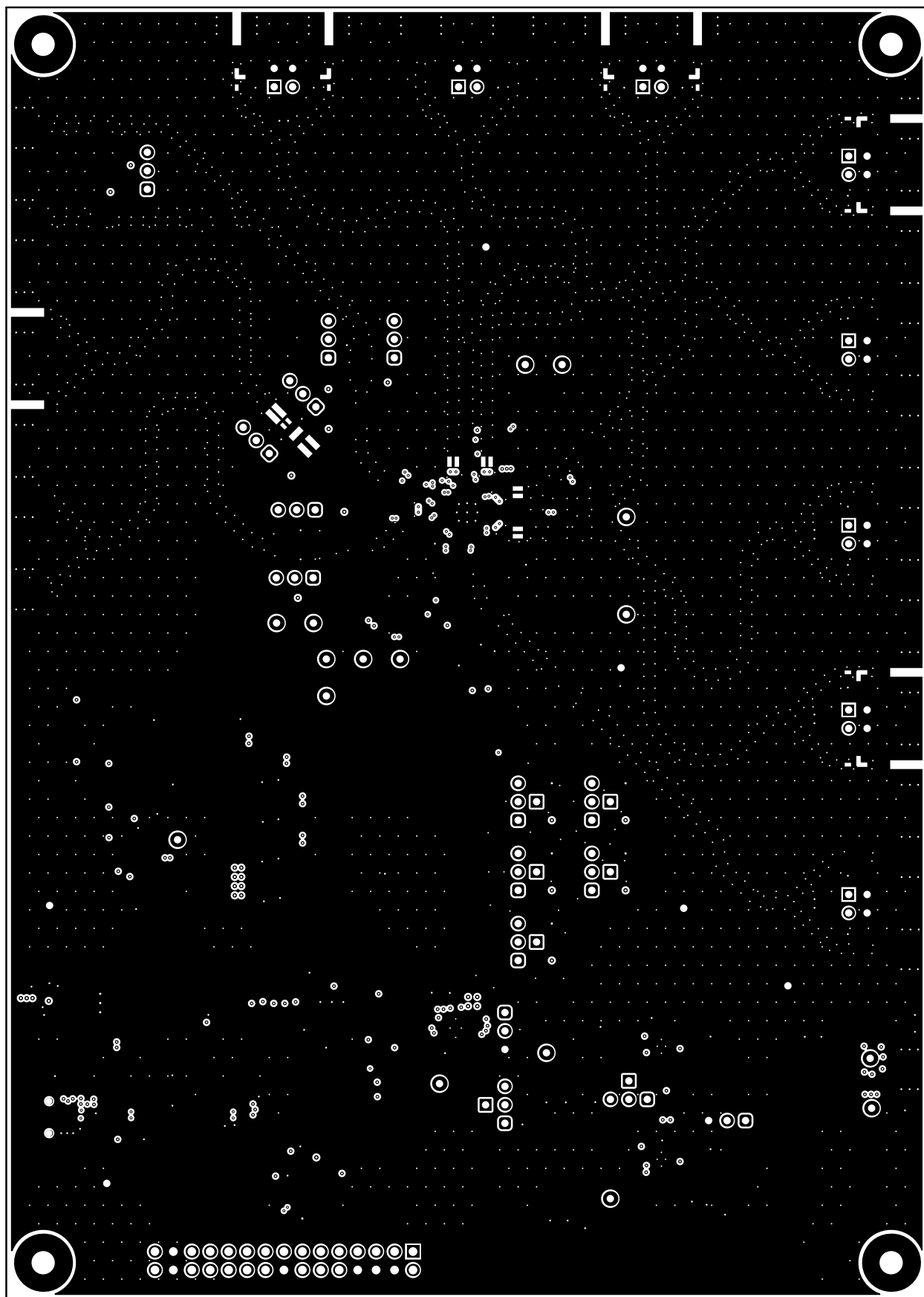
Figure 5-13. LMK3H2108EVM Signal Layer 4
