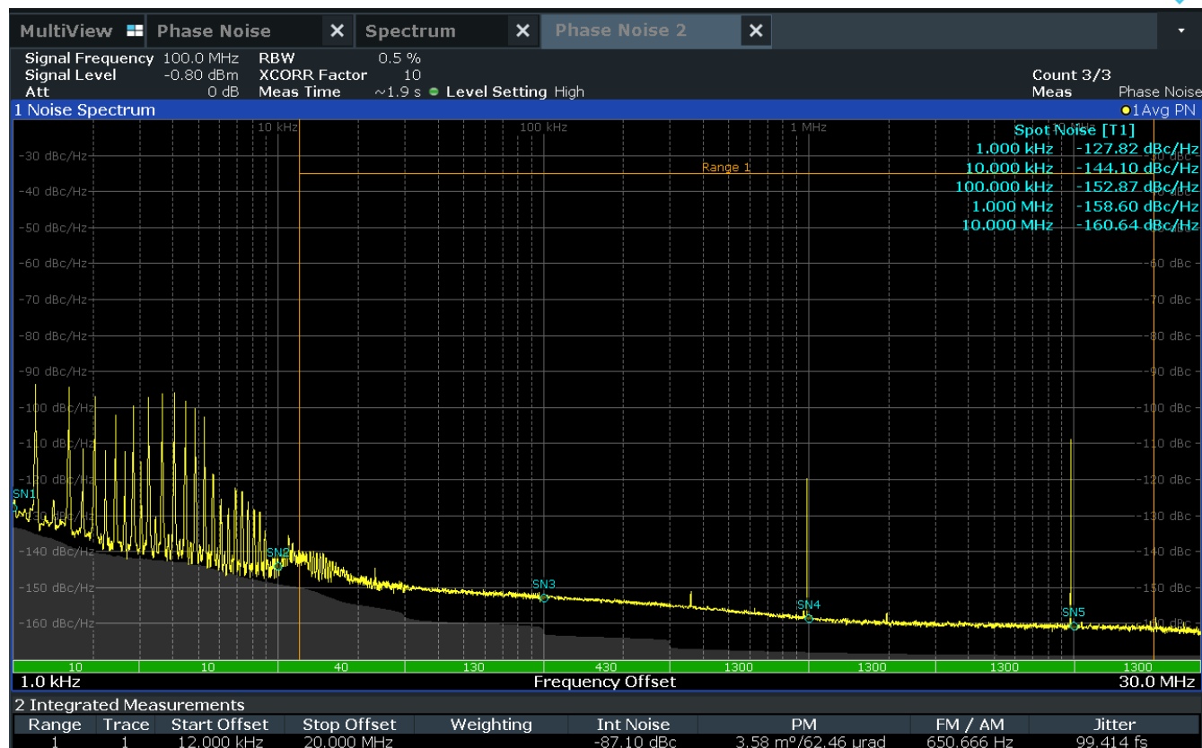
Figure 4-3. LMK3H2108 Typical Performance in Buffer Mode, SMA100B 100MHz Input
