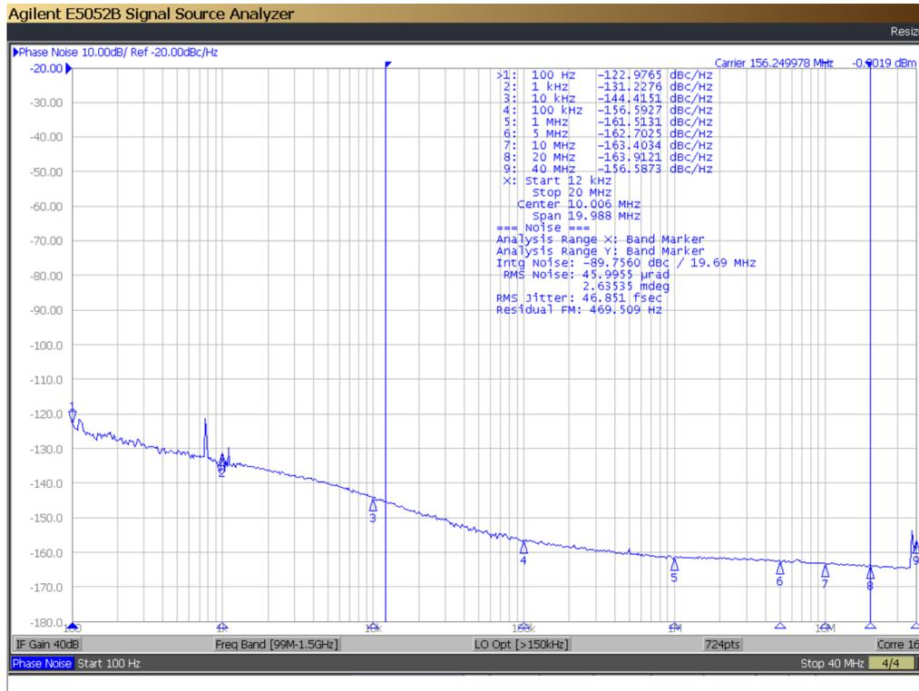
Figure 5-1. LMKDB1104 Output Clock Phase Noise
