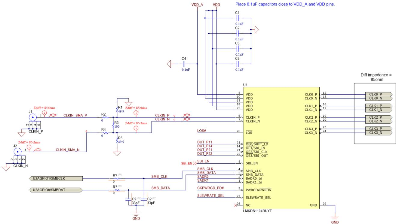
Figure 6-2. LMKDB1104 Device and CLKIN\_P/N Reference
