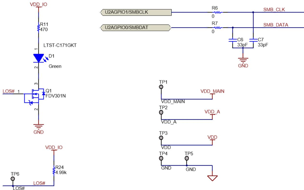
Figure 6-6. Status LEDs, Test Points, and SMBus Clock and Data Connections
