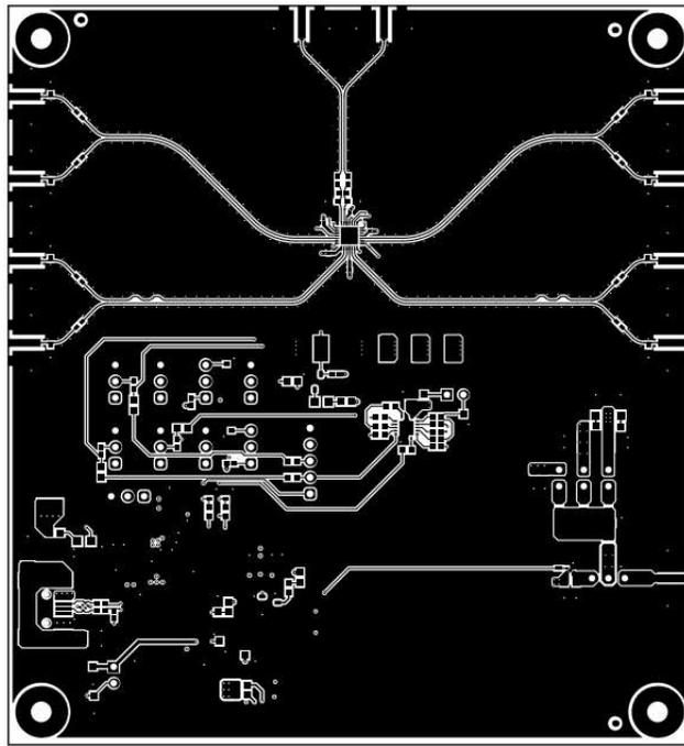
Figure 6-9. Top Layer (CLKIN / CLKOUT Signals)
