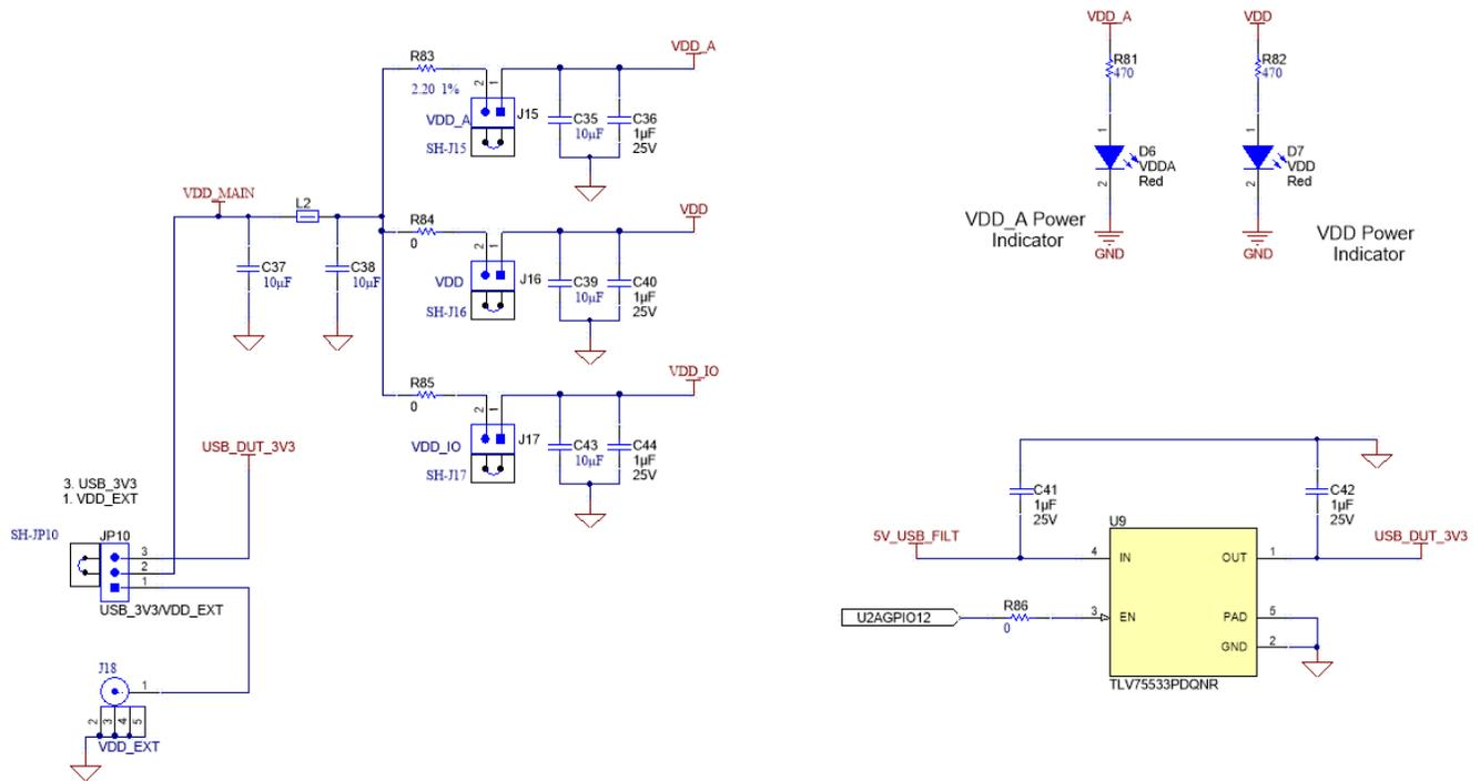
Figure 6-1. Power Supply (External and USB option)
