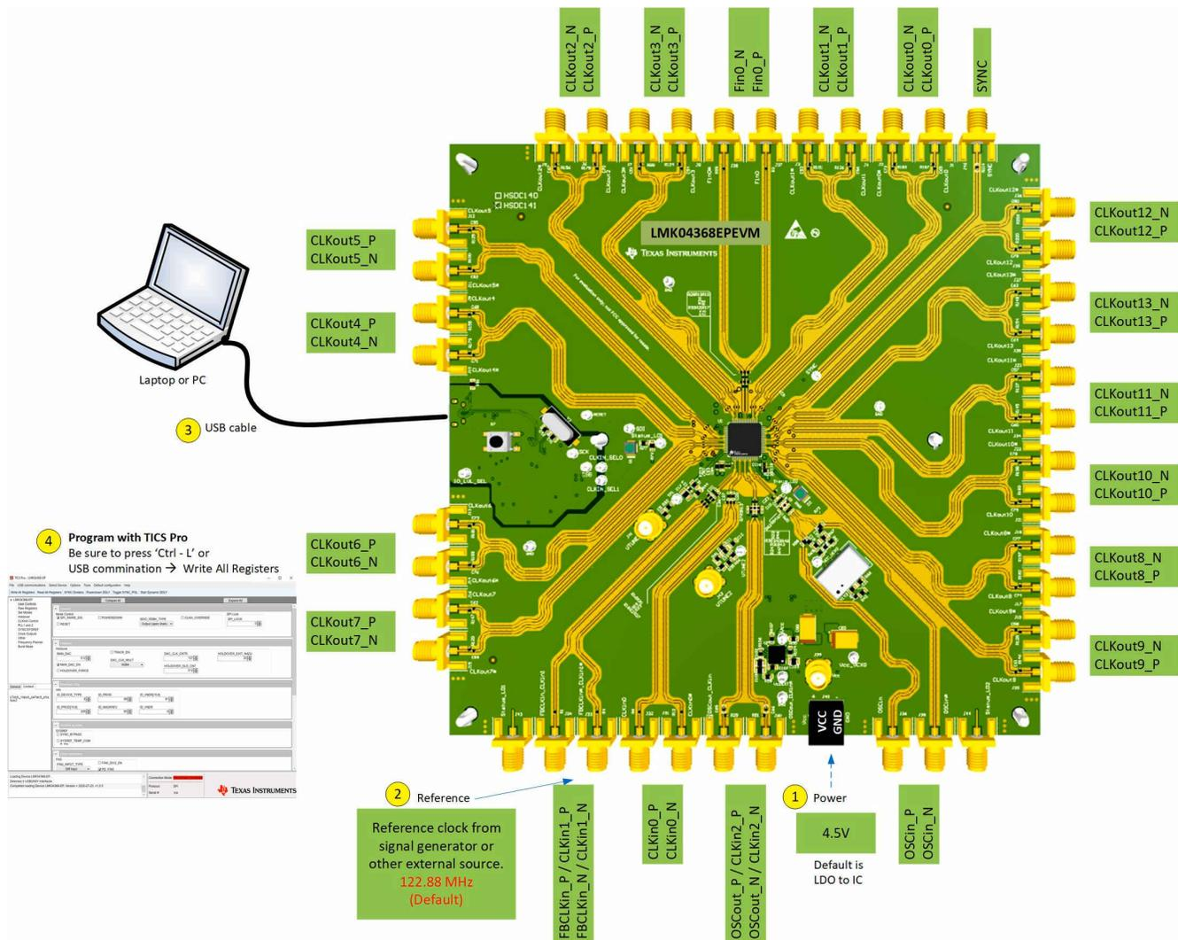
**Figure 2-1. Quick Start Diagram**
