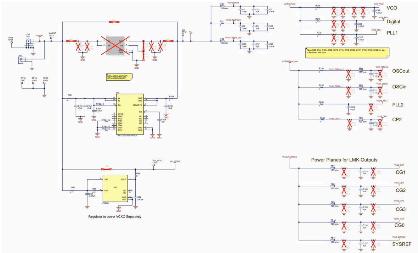
Figure 8-2. Schematic - Power Supply
