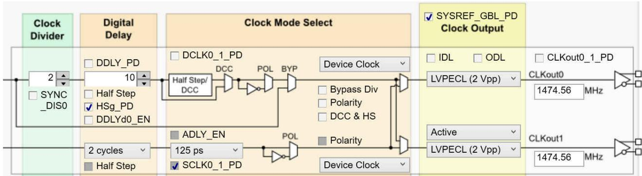
**Figure 5-4. Setting Digital Delay, Clock Divider, Analog Delay, and Output Format**
