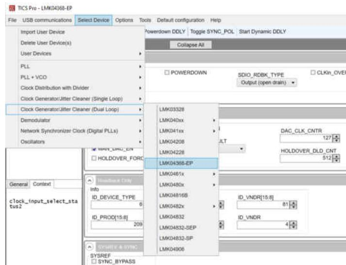
Figure 5-1. Selecting the LMK04368-EP
