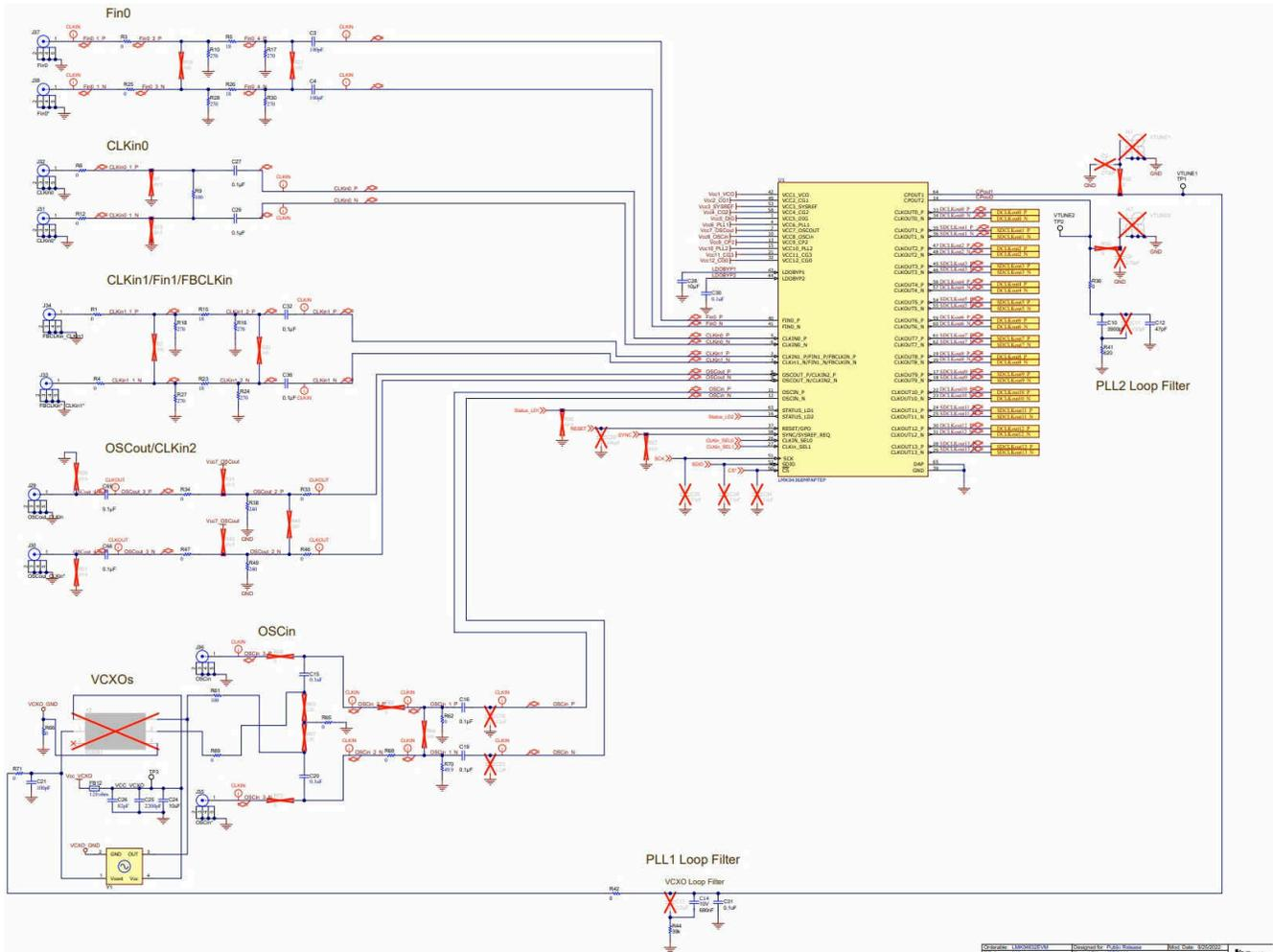
Figure 8-1. Schematic - LMK04368-EP
