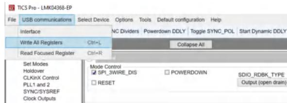
Figure 5-2. Loading the Device
