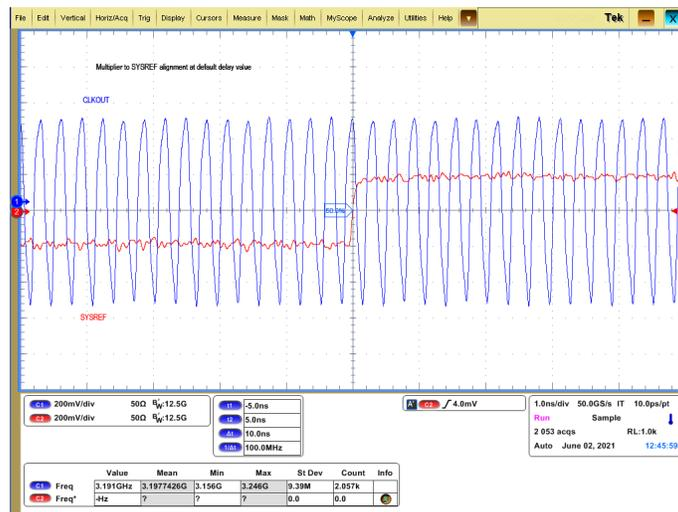
**Figure 3-6. 3200-MHz Multiplier Mode With CLKOUT, LOGICLK, and SYSREF**
