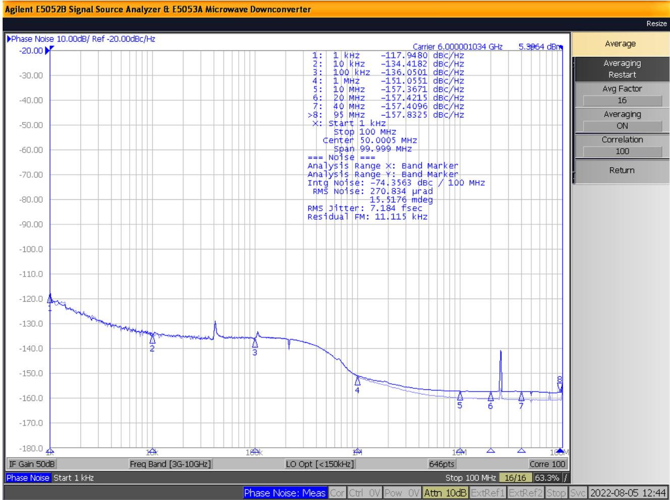
Figure 3-2. 6000-MHz Buffer Mode Signal Analyzer Plot
