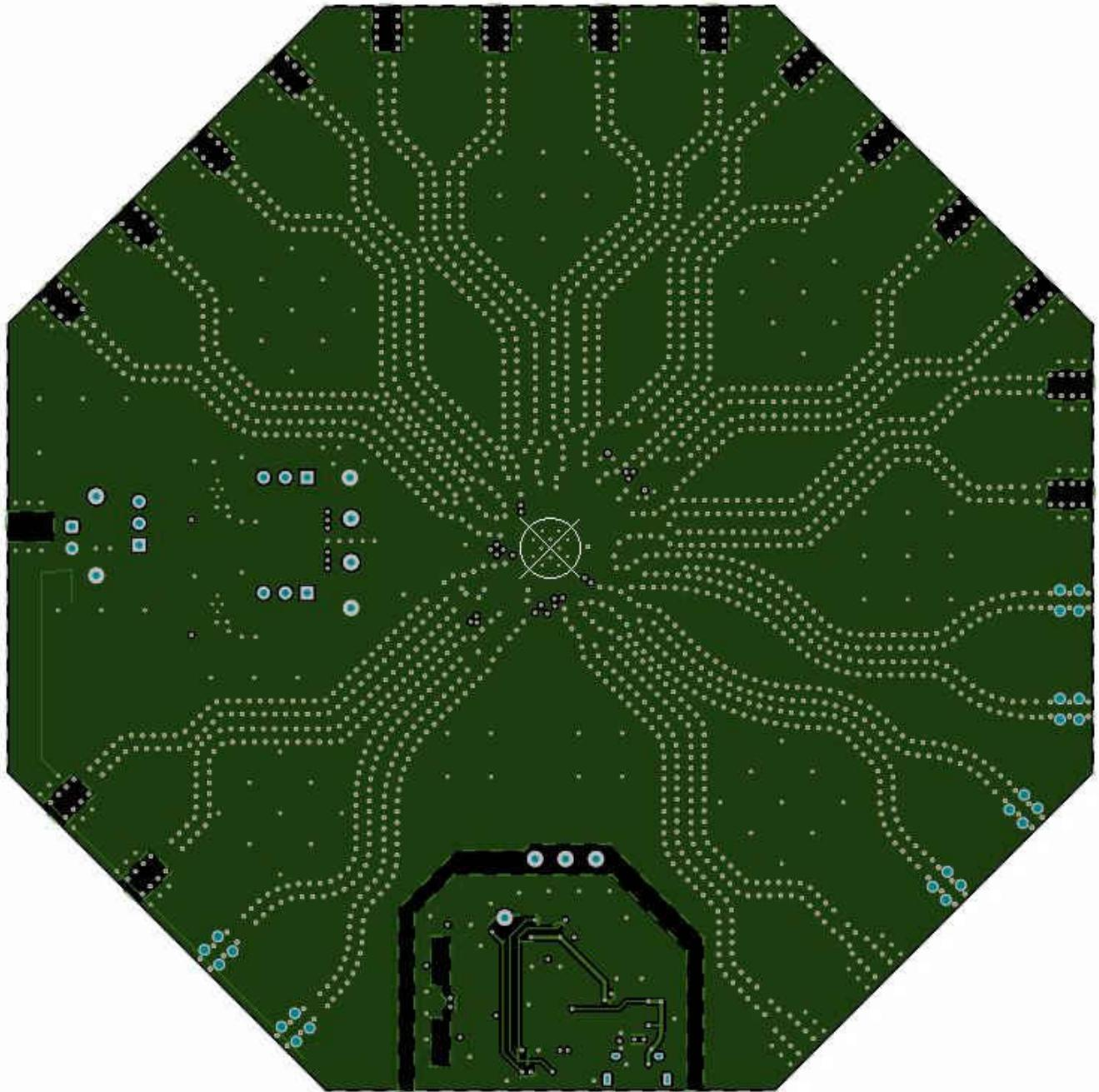
**Figure 5-3. PCB Layer Plot - Layer 2 (RF GND)**
