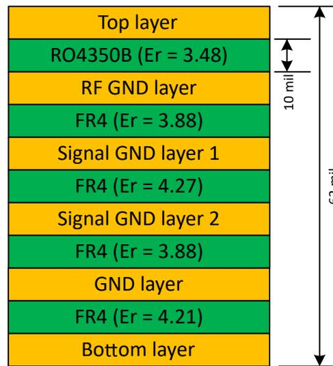
Figure 5-1. PCB Layer Stack-Up
