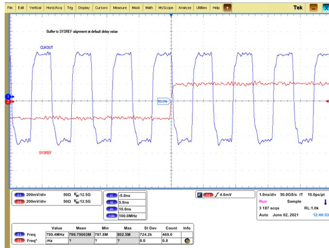
**Figure 3-5. 800-MHz Buffer Mode With SYSREF**
