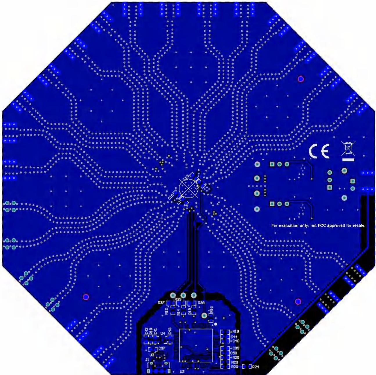
Figure 5-7. PCB Layer Plot - Bottom Layer
