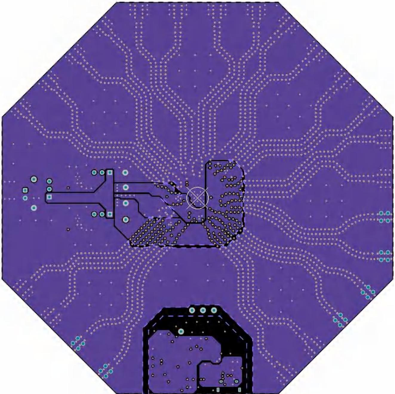
**Figure 5-5. PCB Layer Plot - Layer 4 (Signal GND 2)**
