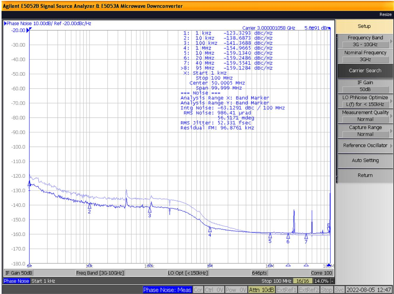
Figure 3-3. 3000-MHz Divide-by-2 Mode Signal Analyzer Plot
