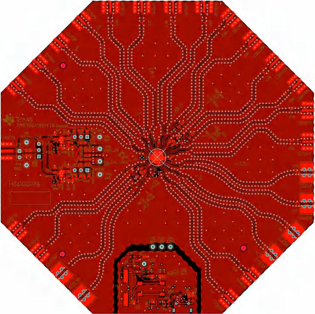
Figure 5-2. PCB Layer Plot - Top Layer
