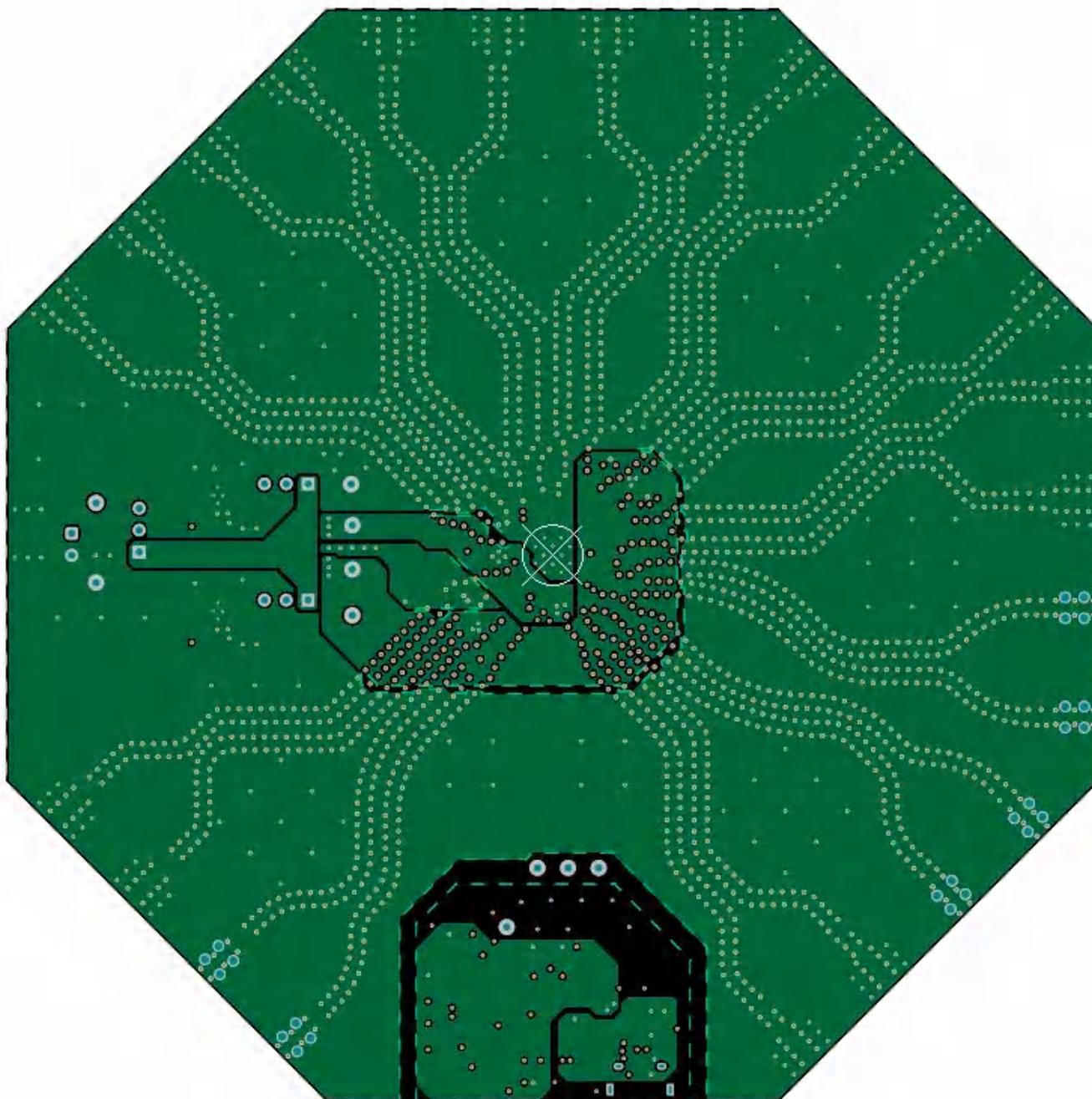
**Figure 5-4. PCB Layer Plot - Layer 3 (Signal GND 1)**
