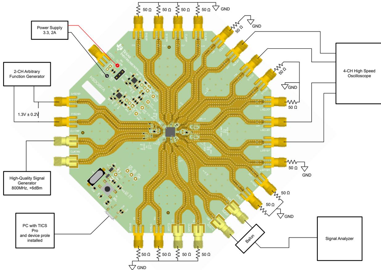
**Figure 2-1. EVM Connection Diagram**
