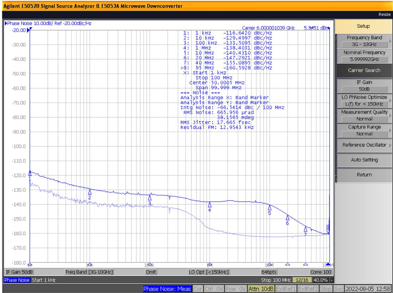
Figure 3-4. 6000-MHz Multiplier x2 Mode Signal Analyzer Plot
