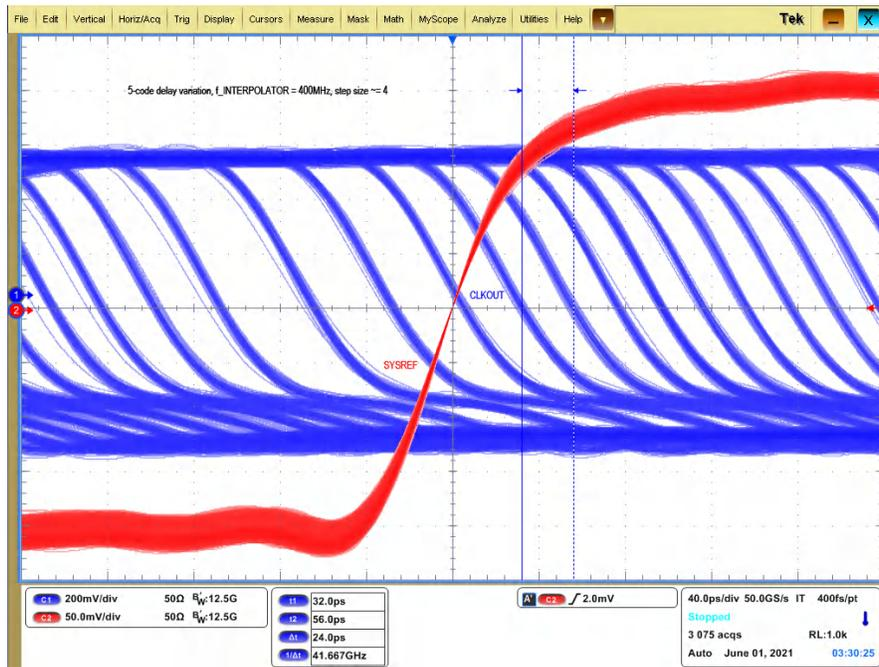
Figure 3-7. SYSREF Delay, in 5-Code Steps
