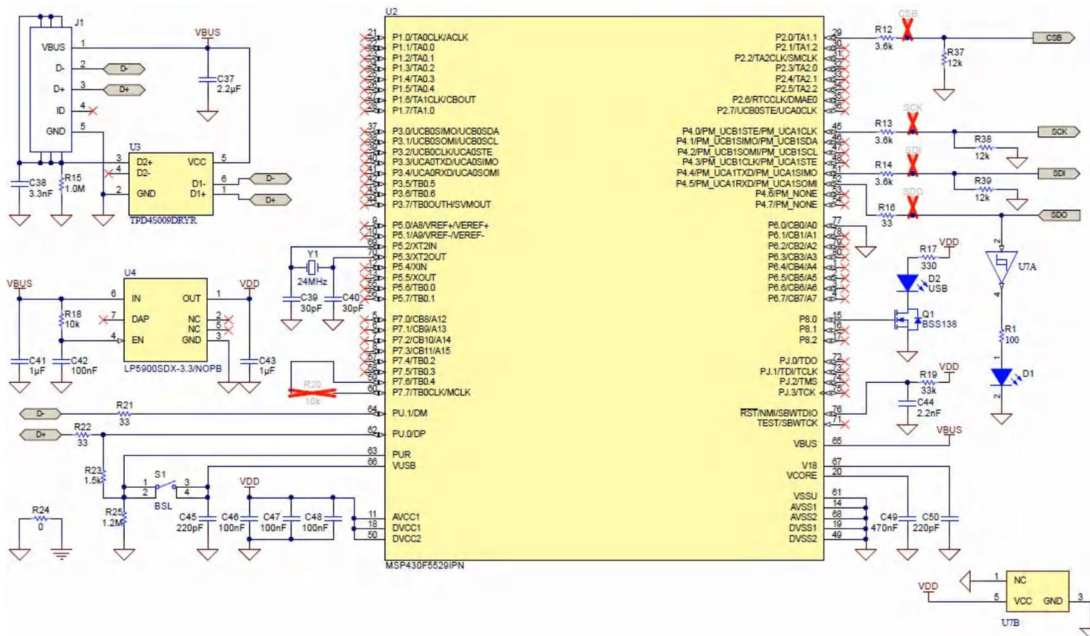
Figure 4-2. Schematic - LMX1204
