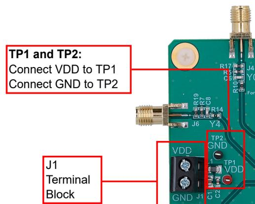
**Figure 4-1. Power Supply Connection Locations**
