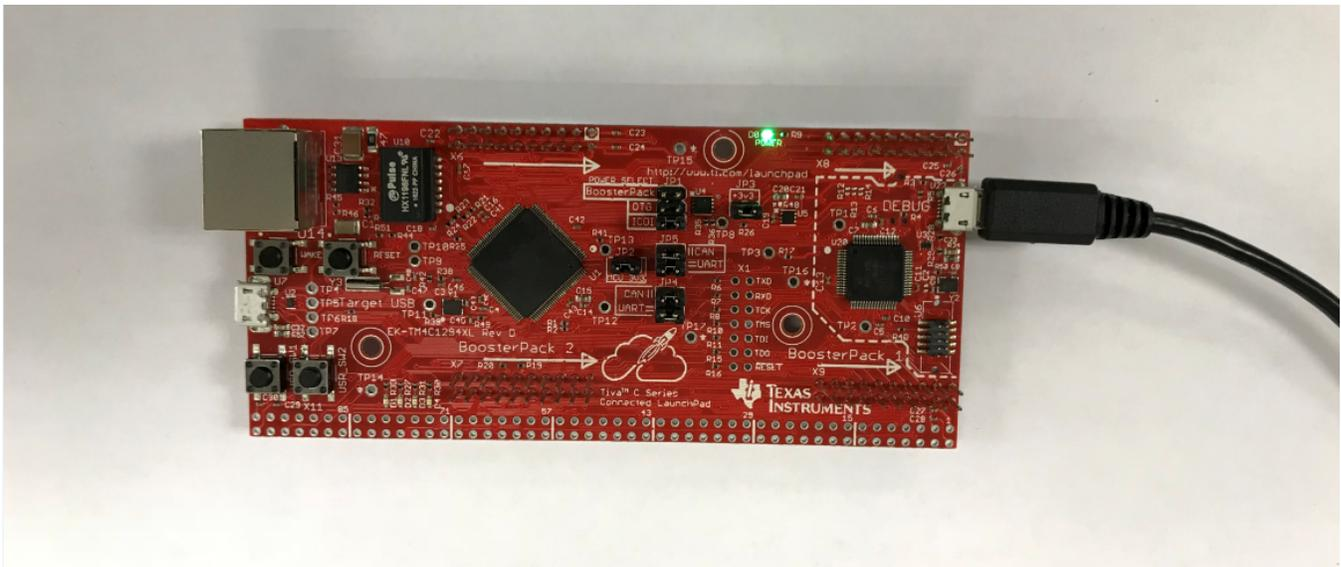
**Figure 6. TM4C1294 LaunchPad™ Software Programming Setup**
