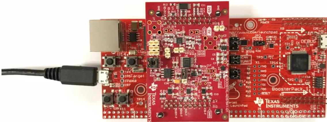
**Figure 10. BOOSTXL-ADS7841-Q1EVM stacked on TM4C1294 LaunchPad™**
