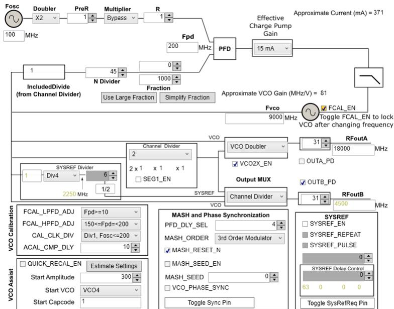
Figure 22. VCO Frequency Doubler Setup in TICSPRO
