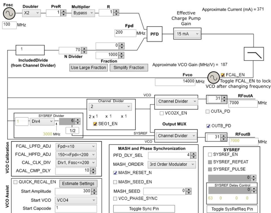
Figure 7. TICS Pro GUI LMX2595 Default Configuration
