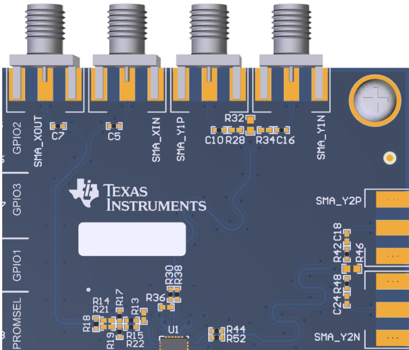
Figure 2-4. Rework, Input, and Output Termination Options
