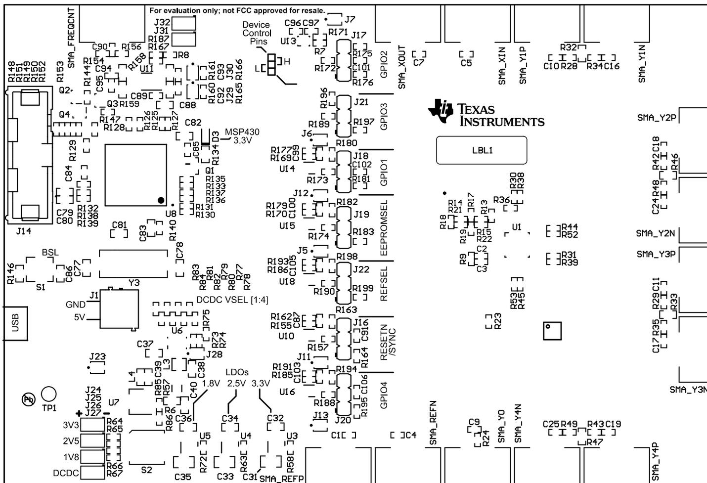
Figure A-10. Layout, Assembly Top
