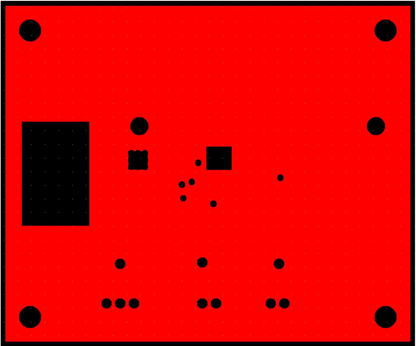
Figure 5-3. GND Plane (Layer 2)
