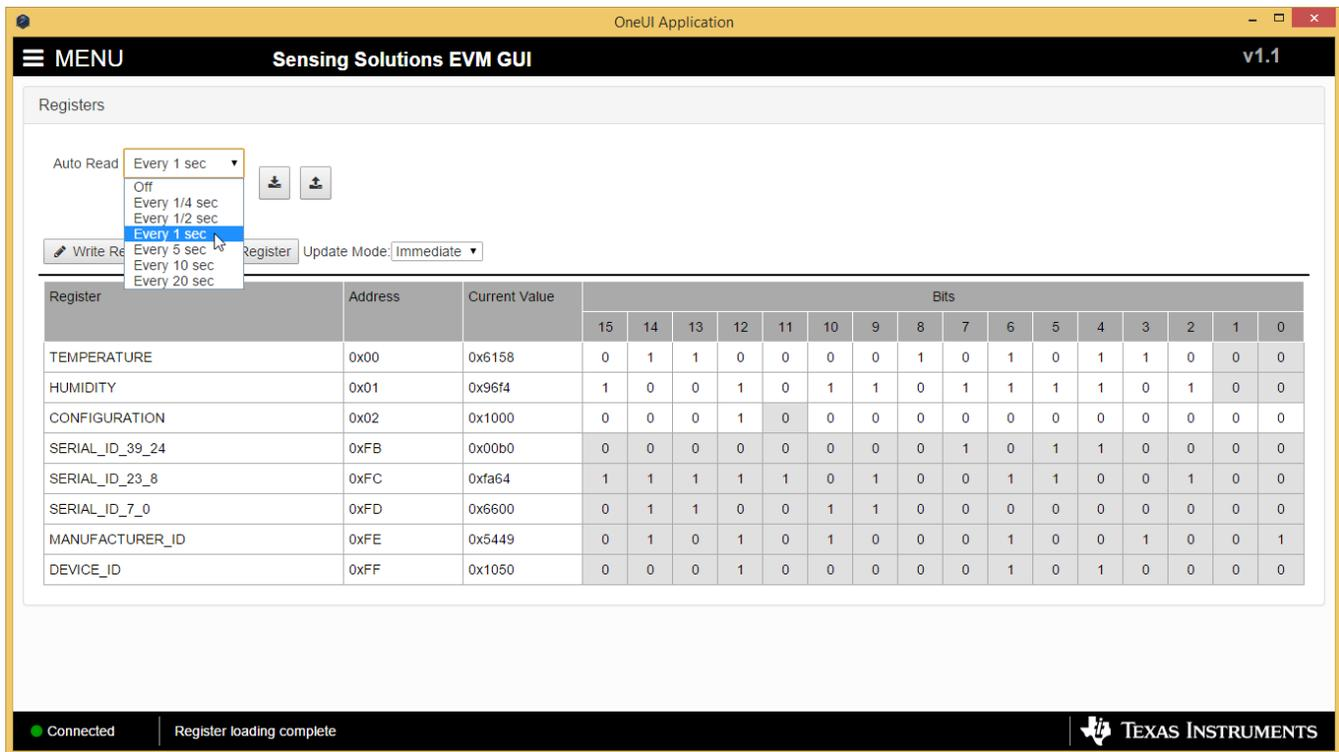
Figure 21. Selecting Auto-Read Interval on Register Page
