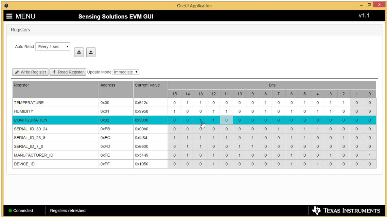
Figure 26. Toggling Register Bit Value on Register Page
