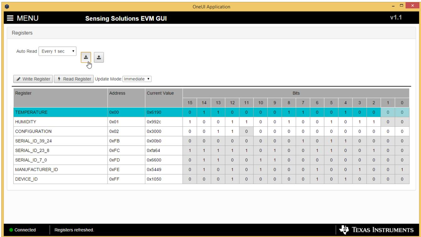
Figure 29. Save Register Values to File on Register Page
