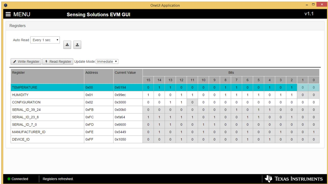
Figure 27. Selecting a Register on Register Page
