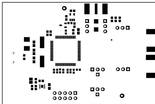
Figure 13. Bottom Solder Mask
