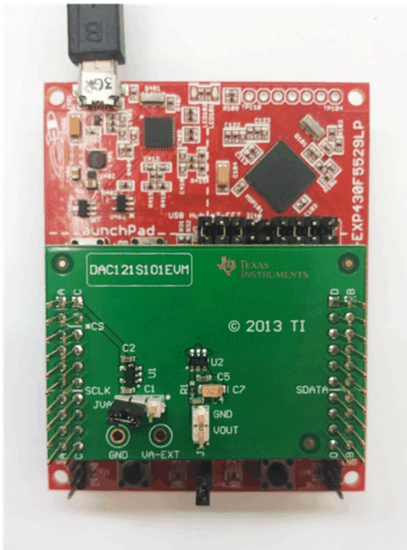
**Figure 3-1. DAC121S101EVM Attached to MSP430**
