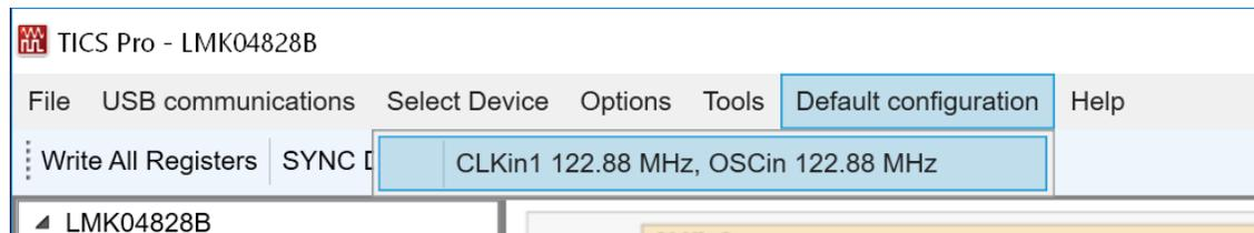
**Figure 6. Selecting a Default Mode for the LMK04828 Device**
