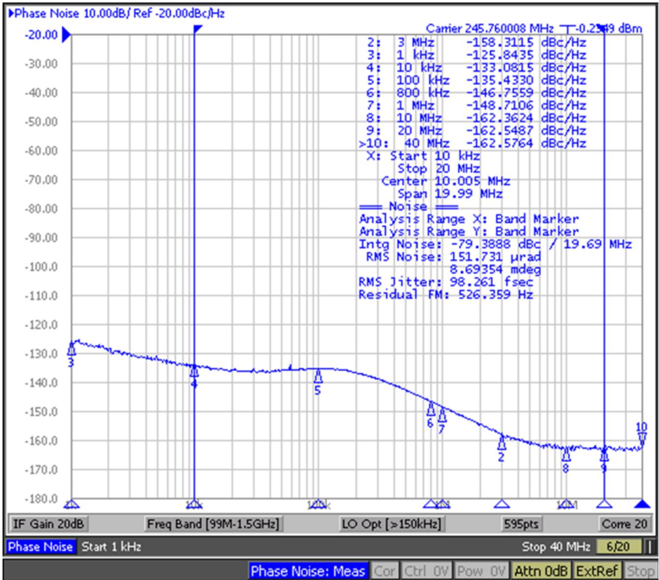
Figure 20. LMK04826 DCLKout2, VCO0, 245.76 MHz, Div8, LVPECL20 /w 240- $\Omega$  Emitter Resistor, DCLKoutX\_MUX=Divider, IDL=1, ODL=0, Balun = Prodyn BIB-100G
