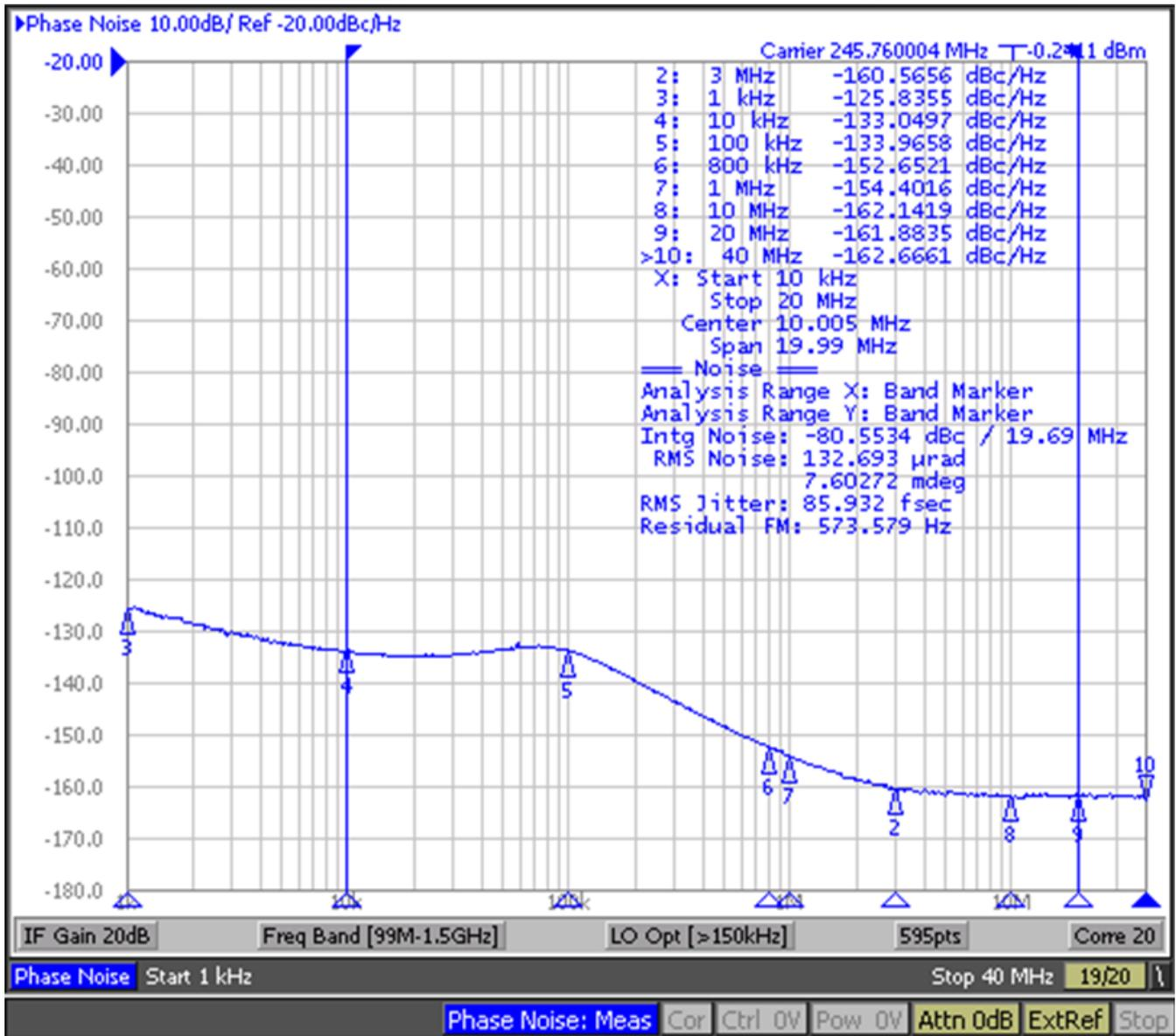
Figure 22. LMK04826 DCLKout2, VCO1, 245.76 MHz, Div10, LVPECL20 /w 240 ohm emitter resistor, DCLKoutX\_MUX=Divider, IDL=1, ODL=0, Balun = Prodyn BIB-100G
