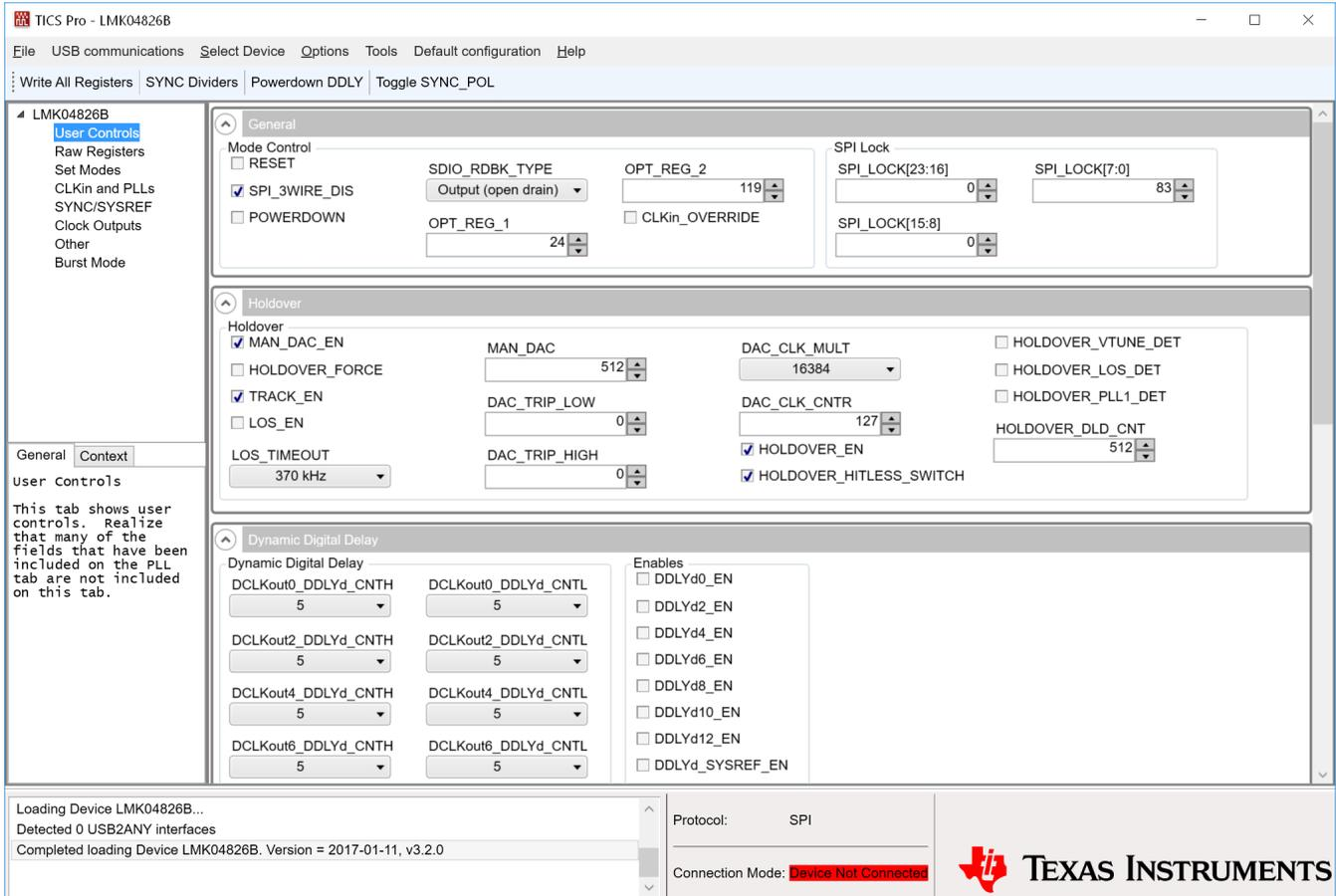
The screenshot displays the TICS Pro software interface for the LMK04826B device. The 'User Controls' tab is active, showing various configuration options:
