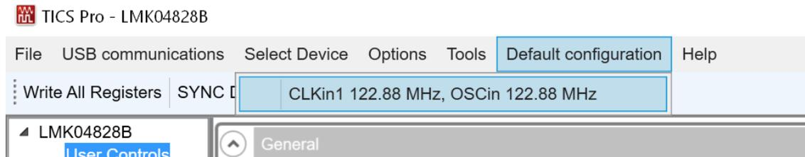
**Figure 9. Setting the Default Mode for LMK04828**
