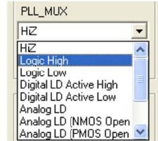
Figure 9 - Programming the PLL\_MUX of the LMK03000C.
