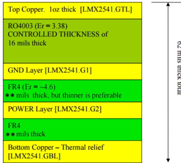
**Figure 3-1. Board Stackup Parameters**
