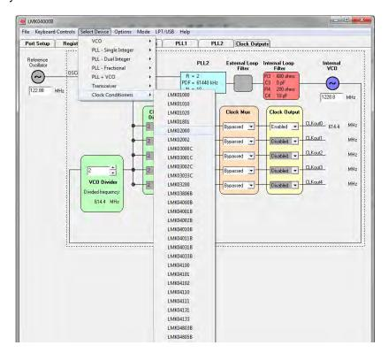
6) Enable the output to measure (example CLKout0 is enabled below)
