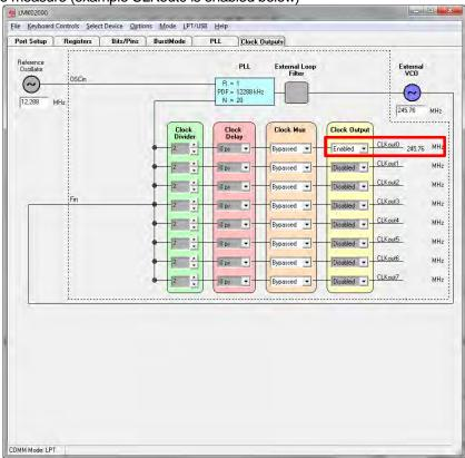
7) **Program** the part by clicking "Keyboard Controls" → "Load Device" or by pressing Ctrl+L.
