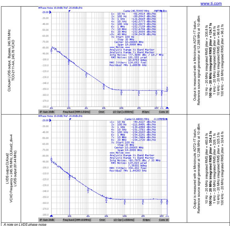
LVDS drivers expect a 100 ohm differential load for optimal phase noise performance. We recommended that a balun be used when making single ended (unbalanced) measurements (like the phase noise measurements above).
